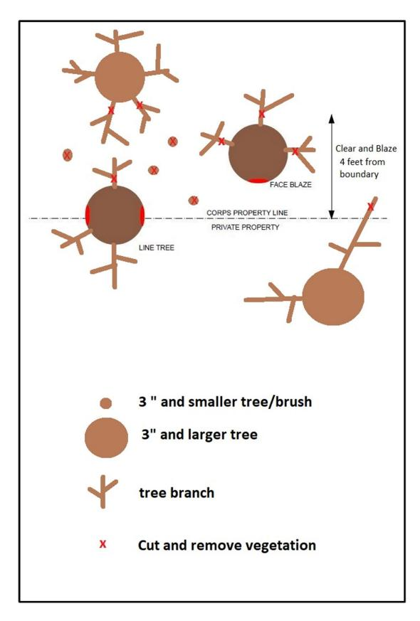
**FIGURE NO 1: Boundary Clearing Specifications**
