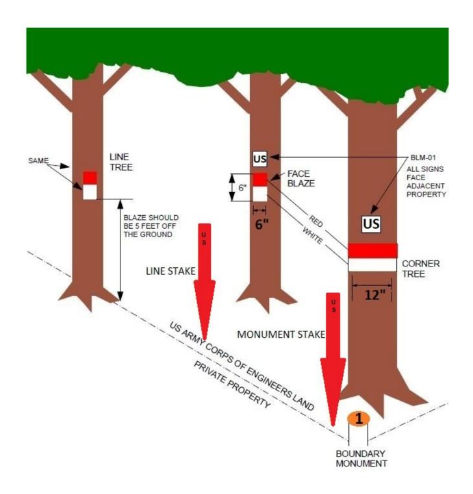
FIGURE NO 2: Boundary Marking Specifications
