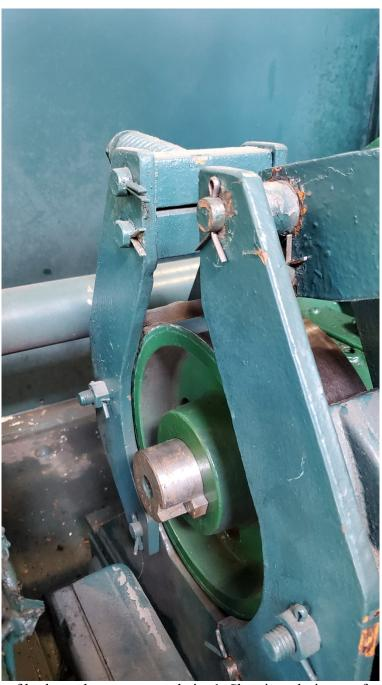
**Photo 8:** Side view of brake and rotor on gate hoist 1. Showing glazing on face of rotor and wear on the size of the rotor due to movement in the armature shaft
