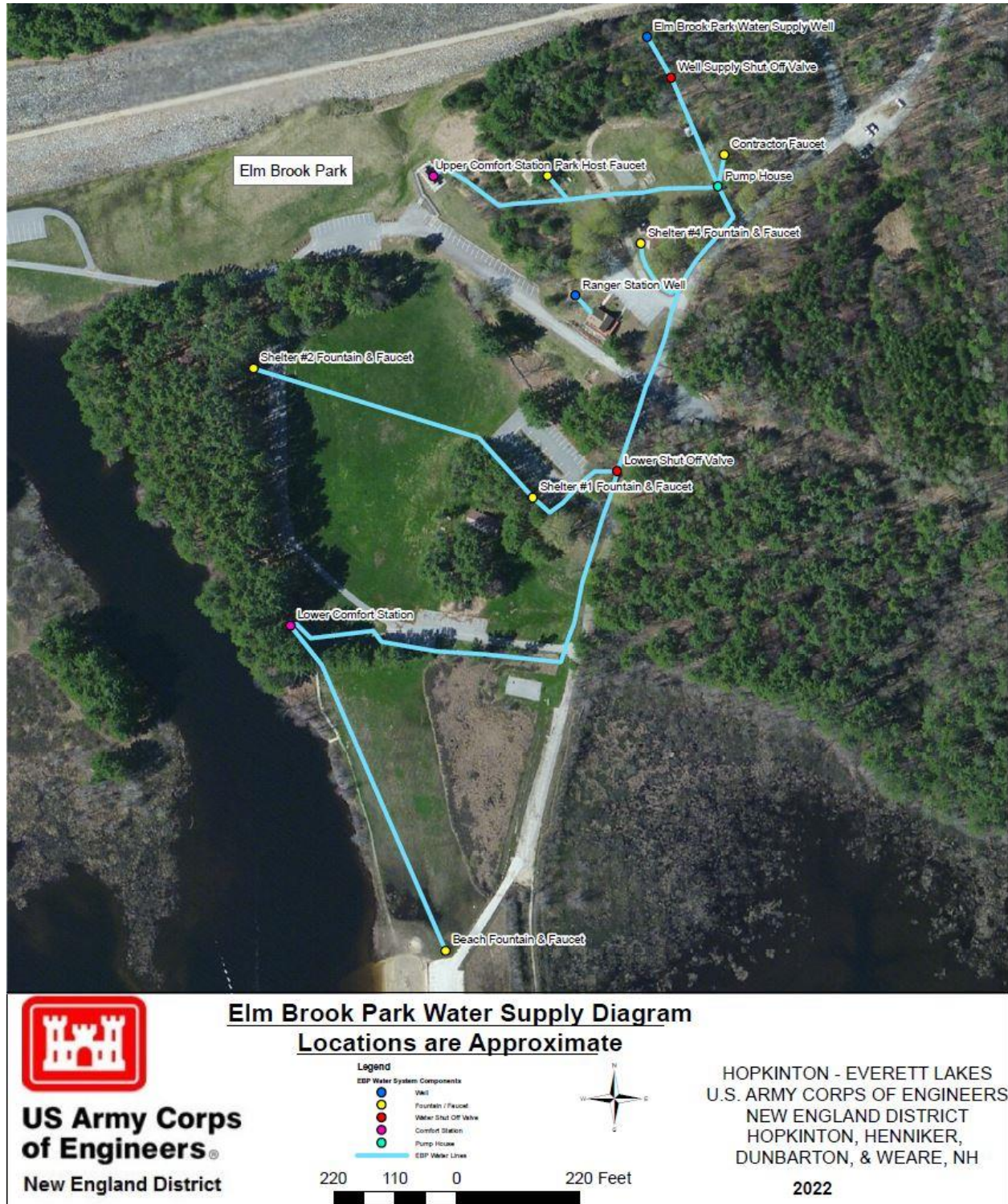
Exhibit 1: Approximate Elm Brook Park waterline schematic.
