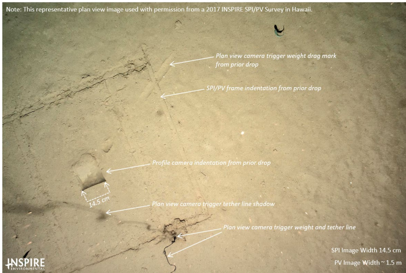
Figure 2-3. This representative plan view image shows the sampling relationship between plan view and sediment profile images. Note: plan view images differ between surveys and stations and the area covered by each plan view image may vary slightly between images and stations.
