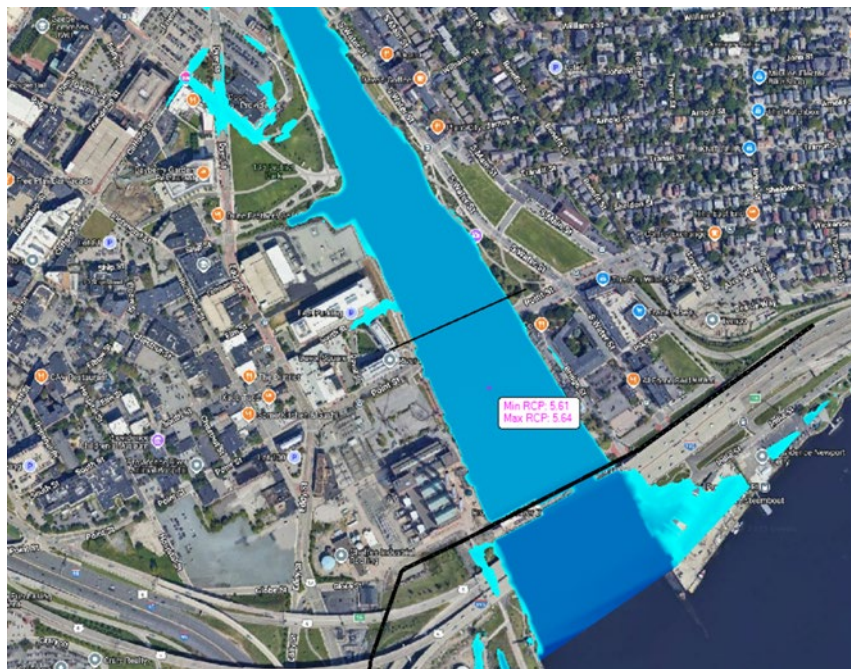
Figure 29. Stage comparison near the barrier: 500-year minimum RCP 8.5 estimate vs. 500-year maximum RCP 8.5 estimate.
