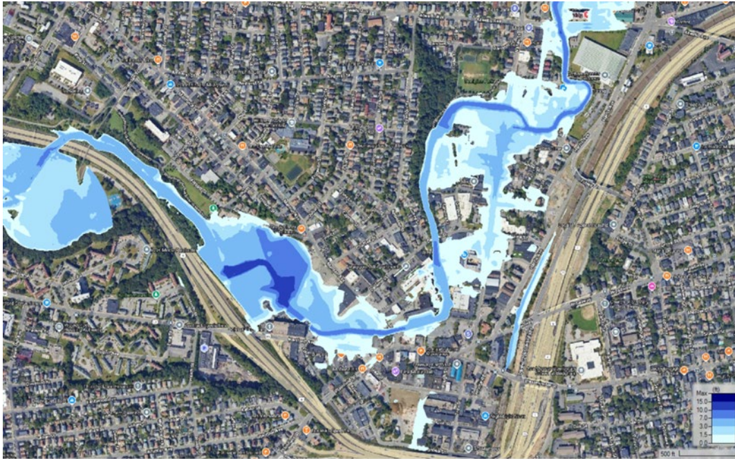
Figure 26. Valley Street and Westminster Steet inundation from a 24-hour 100-year event with the maximum predicted future rainfall increase (RCP 8.5).
