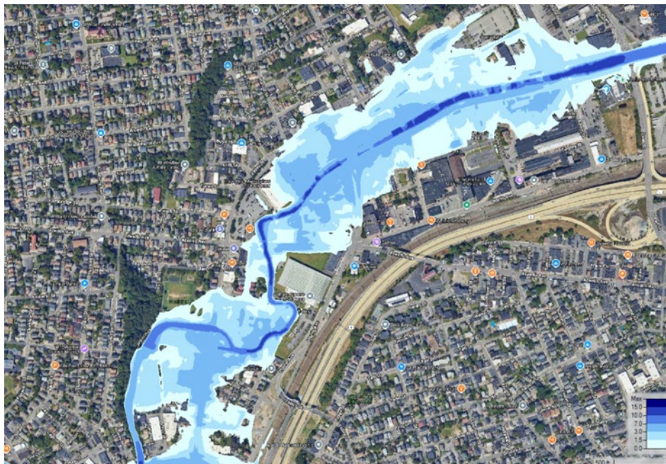
Figure 25. Atwells Avenue inundation from a 24-hour 500-year event with the maximum predicted rainfall increase (RCP 8.5).
