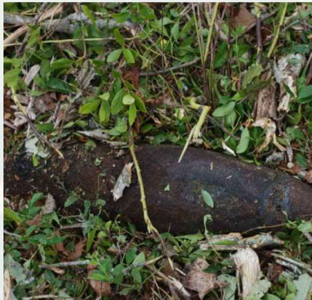
5-inch High Velocity Aerial Rocket MK6 Series (Practice) found during the Remedial Investigation
