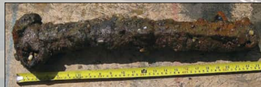
An encrusted rocket motor found at South Beach
