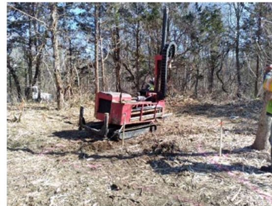
SCENE: View of the Geoprobe Direct Push Technology machine set up at a Boiler House No. 4 (BH4) boring location. DATE: 03 March 2021
