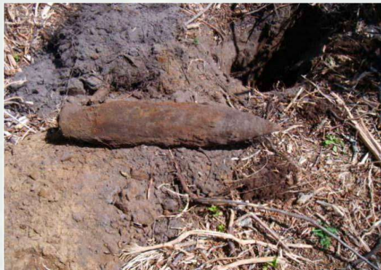
5-inch MK1 Rocket Warhead found during the Remedial Investigation
