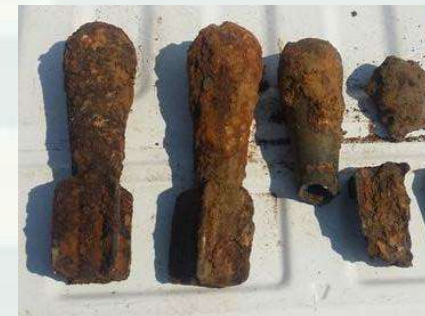
3-lb AN-MK23 Practice Bombs and MD found at the Former Cape Poge Little Neck Bomb Target Site during the Remedial Action
