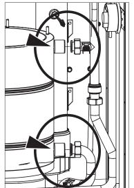
Figure 90 - Remove the CH Supply and Return Pipes
