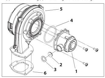
Figure 88 - Removed Fan, Mixer, and Components
