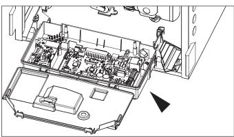
Figure 96 - Disconnect the Main PCB
