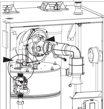
Figure 82 - Remove the gas pipe
