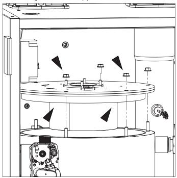
Figure 84 - Remove the Top Plate and Burner
