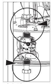
Figure 95 - Disconnect the Gas Valve
