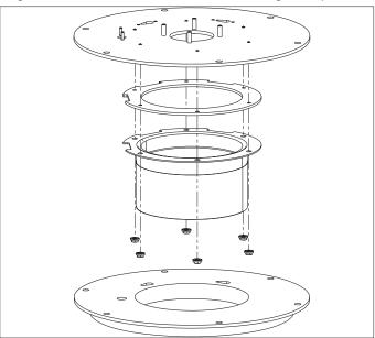
Figure 85 - Disassembled Burner Assembly
