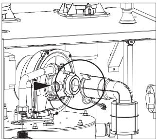
Figure 81 - Remove the silencer
