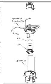
Figure 86 - Clean the Condensate Trap
