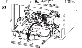
Figure 80 - Removing the Cover and Control Panel Housing Check Water and Gas Piping
