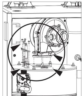
Figure 83 - Remove the Blower and Electrodes
