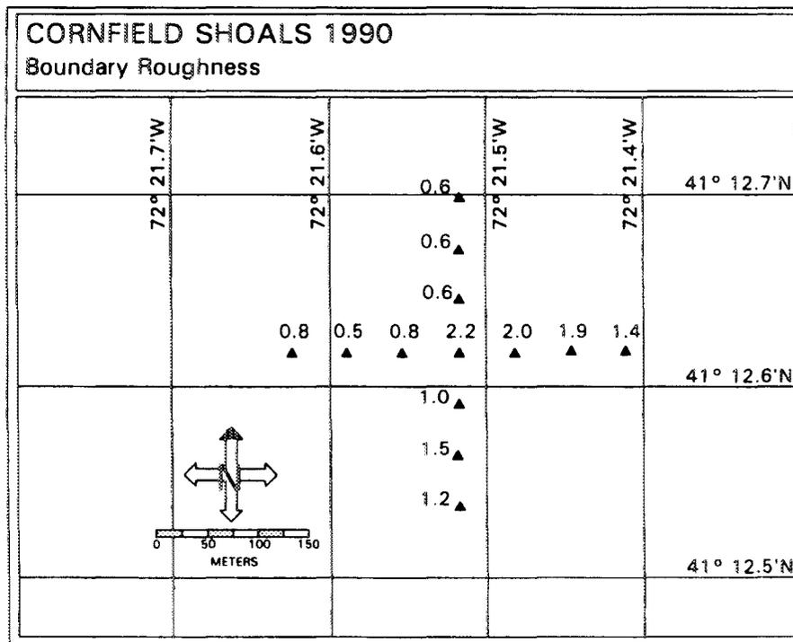
**Figure 3-10.** The mapped small-scale surface boundary roughness values for Cornfield Shoals, 1990.
