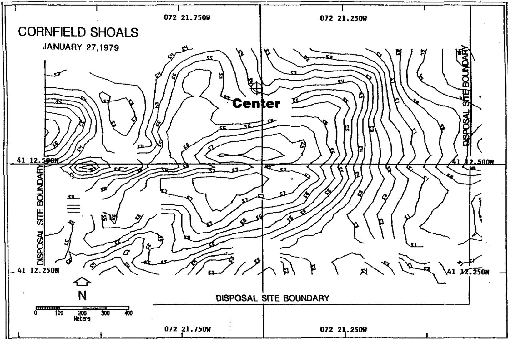
Figure 3-3. Bathymetric contour plot of Cornfield Shoals, January 1979. Contours at 0.5 m intervals.
