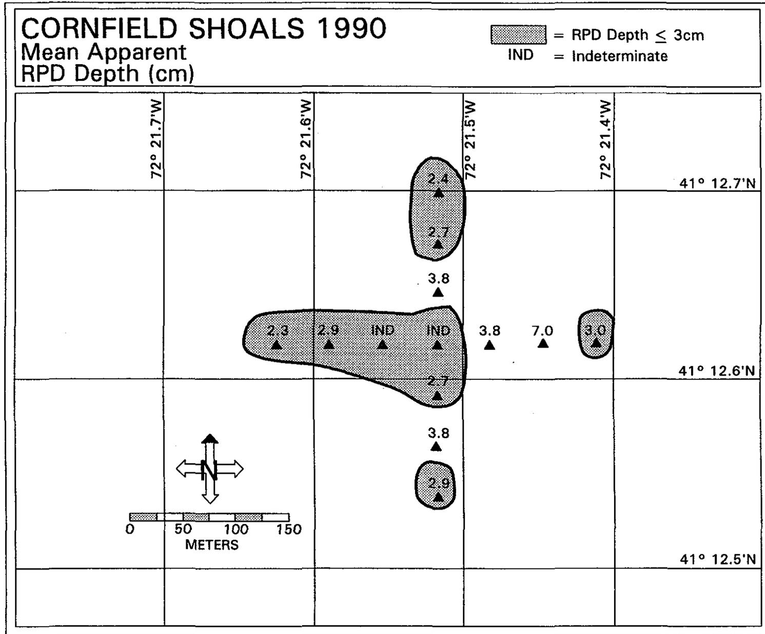
**Figure 3-13.** The distribution of mean apparent RPD depth as determined from the REMOTS® survey at Cornfield Shoals, July 1990. Contour delineates stations where RPD depth  $\leq$  3 cm.
