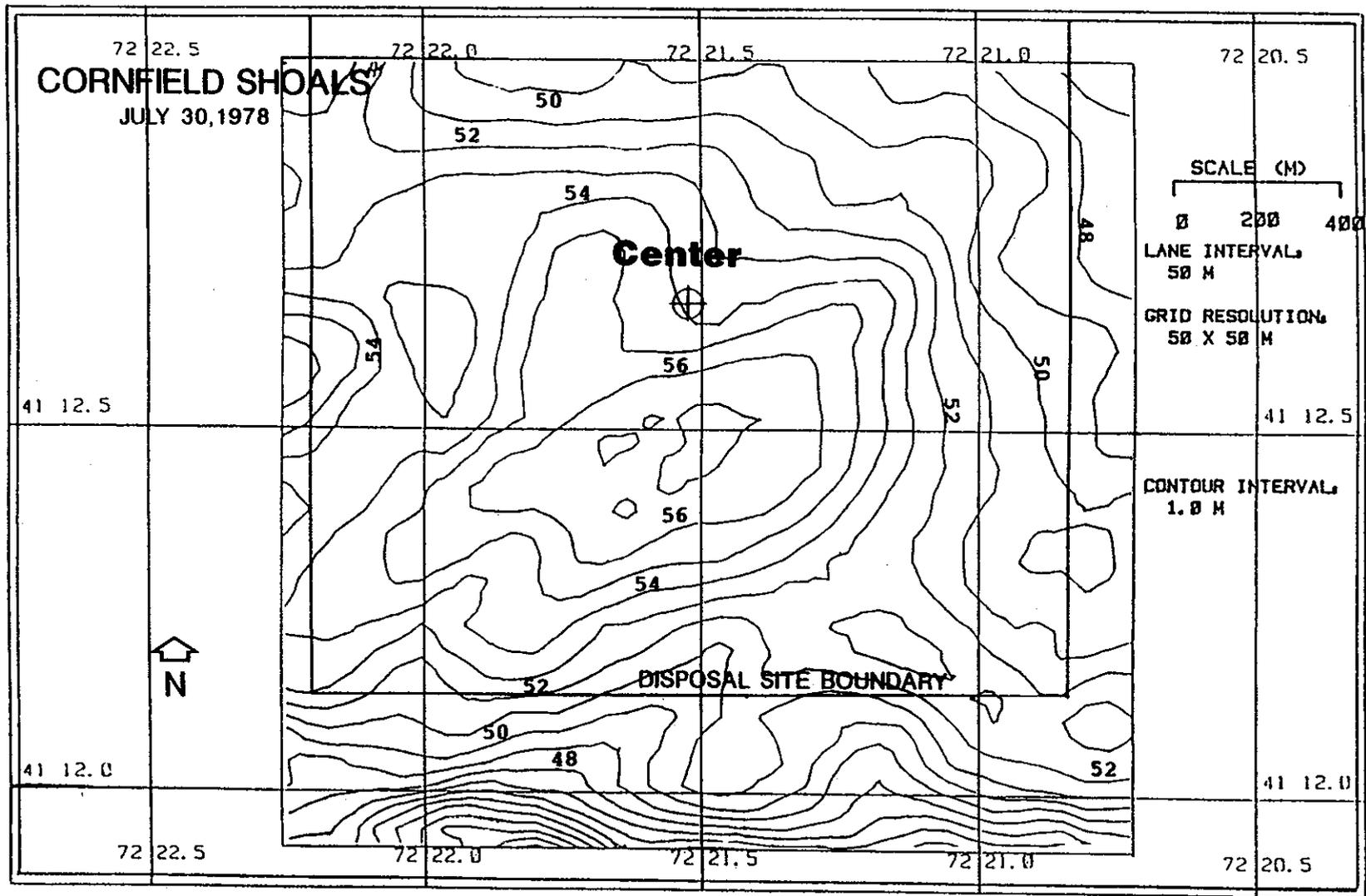
Figure 3-4. Bathymetric contour plot of Cornfield Shoals, July 1978. Contours at 1.0 m intervals.
