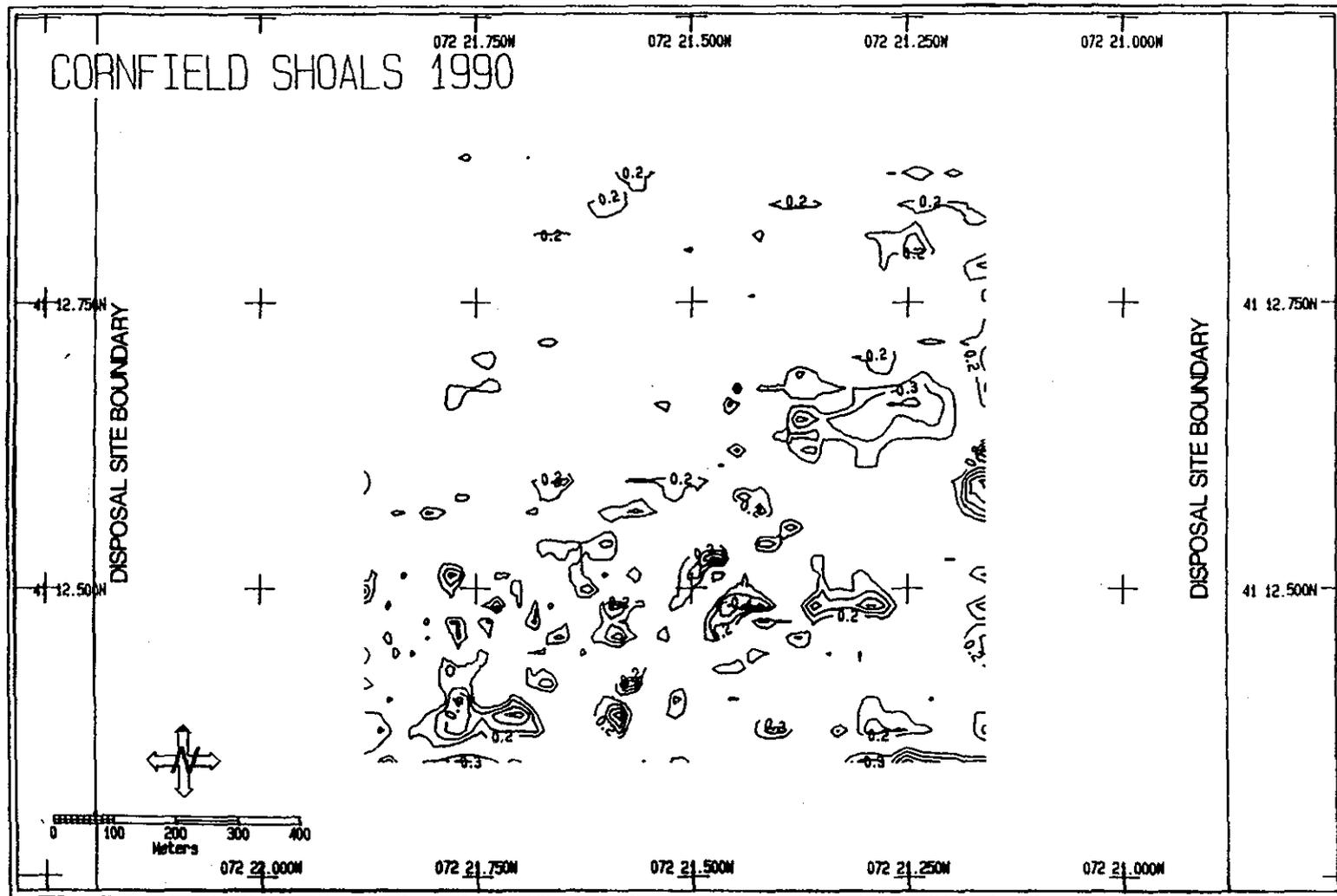
Figure 3-5. Depth difference contour plot of Cornfield Shoals, July 1990. Contours at 0.1 m intervals.
