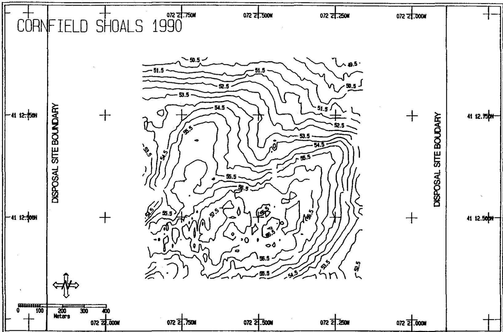
Figure 3-1. Bathymetric contour plot of Cornfield Shoals, July 1990. Contours at 0.5 m intervals.
