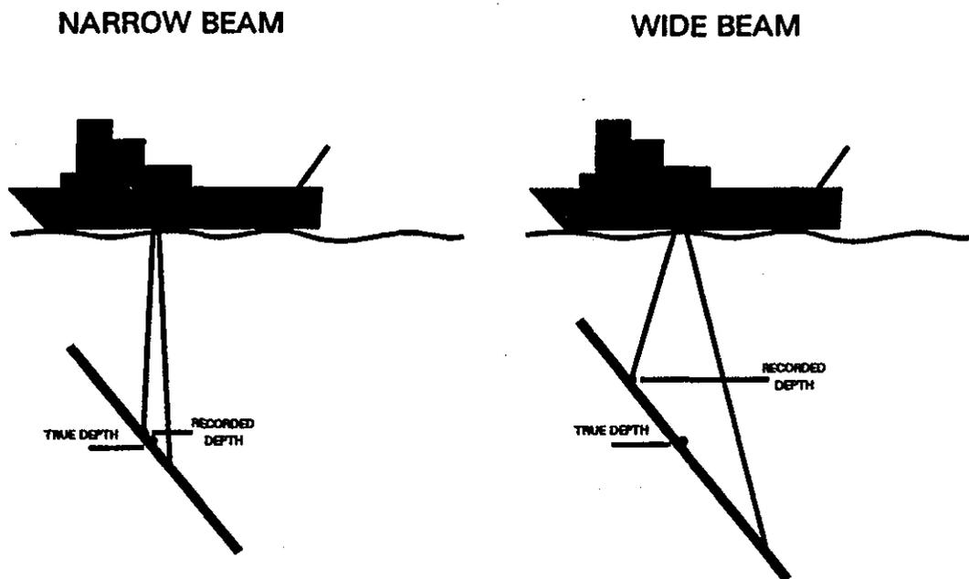
**Figure 3-14.** Changes in transducer beam width can affect the depths recorded during consecutive bathymetric surveys. Notice the apparent decrease in water depth recorded by the "wide beam" transducer.
