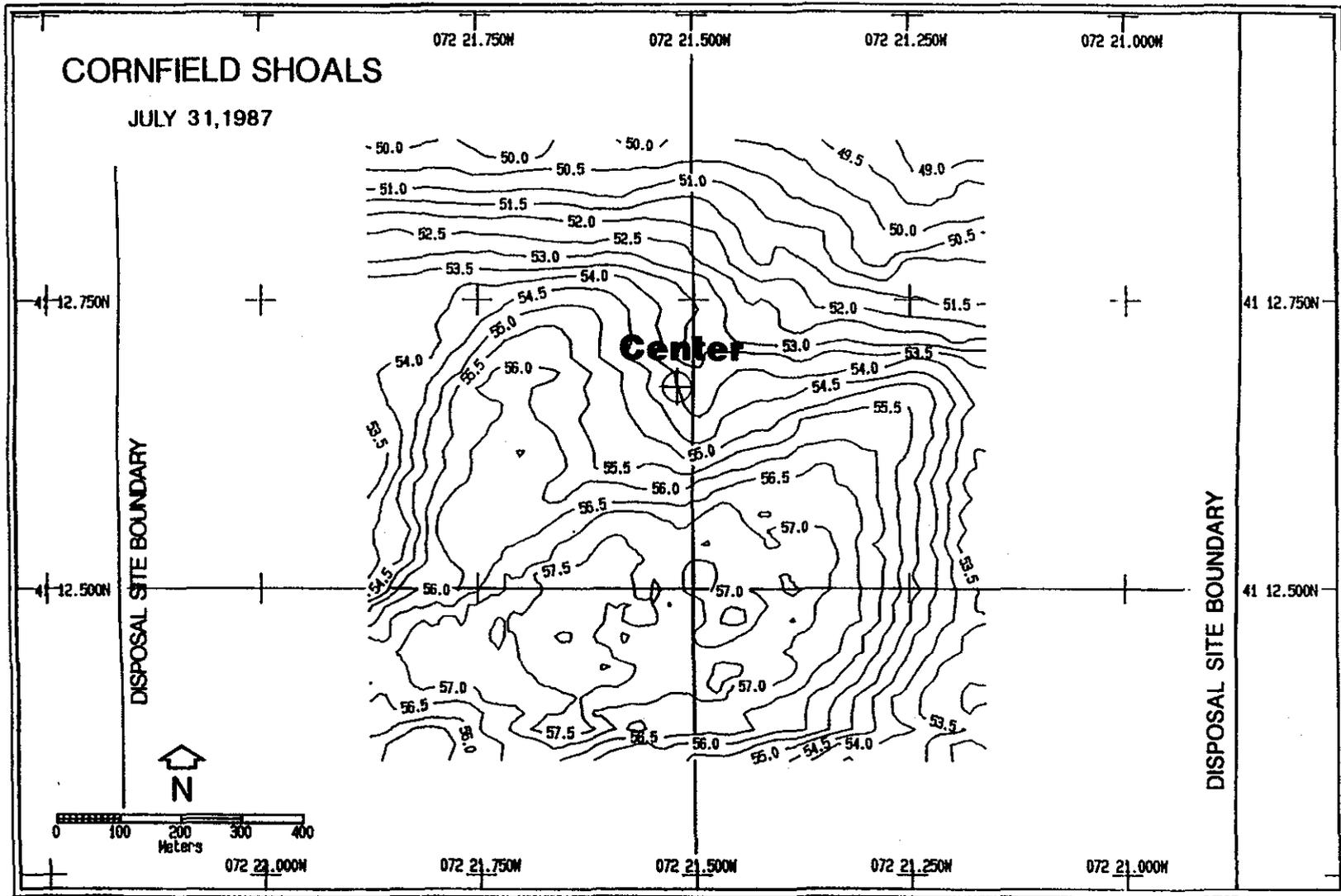
Figure 3-2. Bathymetric contour plot of Cornfield Shoals, July 1987. Contours at 0.5 m intervals.
