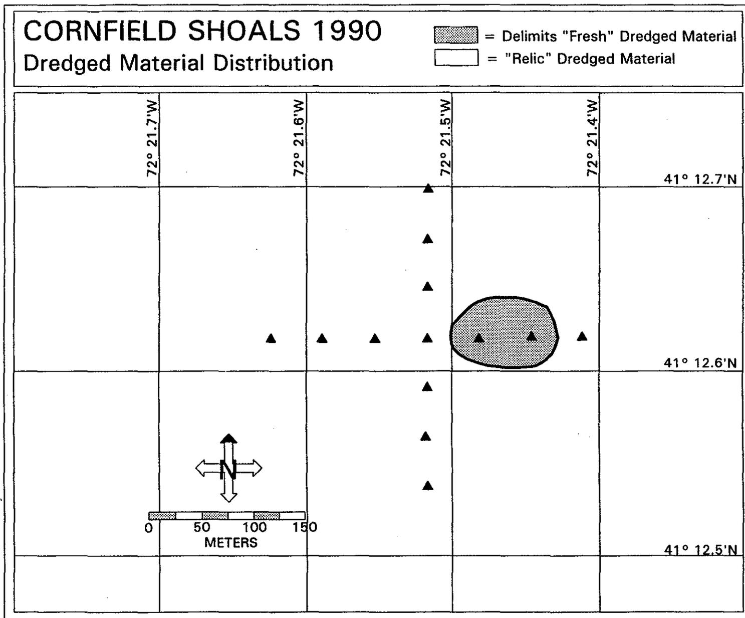
**Figure 3-6.** The mapped distribution of fresh dredged material at Cornfield Shoals, July 1990. The presence of relic dredged material is also indicated.
