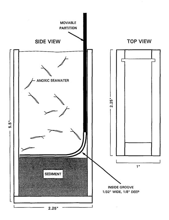
Figure 3-1. Plexiglas sampling box with sliding separator.
