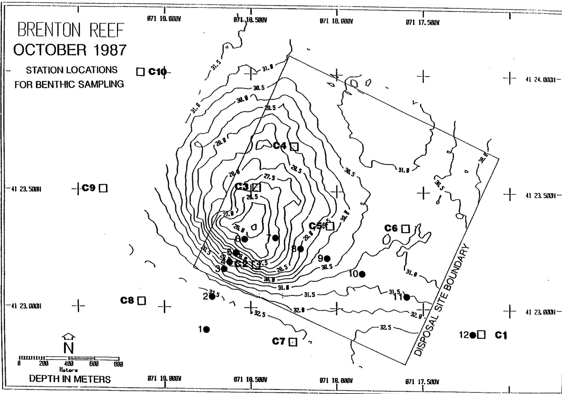
Figure 2-4. Locations of the 10 grab sample stations for grain size and chemical analyses of sediments (stations C1 thru C10 indicated with squares) and locations of the 12 "transect" stations where grab samples for quantitative benthic analyses were obtained (circles) at the Brenton Reef study site in October 1987.
