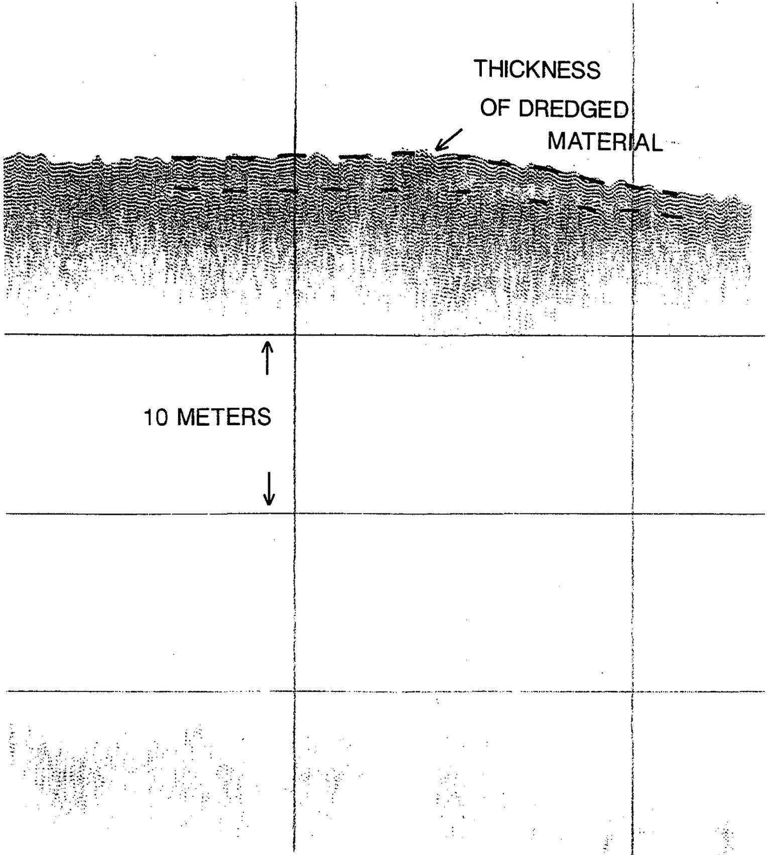
Figure 3-3. A representative seismic profile at the Brenton Reef study site. The historic disposal mound is easily discerned as a surface feature distinct from the original pre-disposal horizon; no distinct sub-bottom acoustic features were noted at or in the vicinity of the mound.
