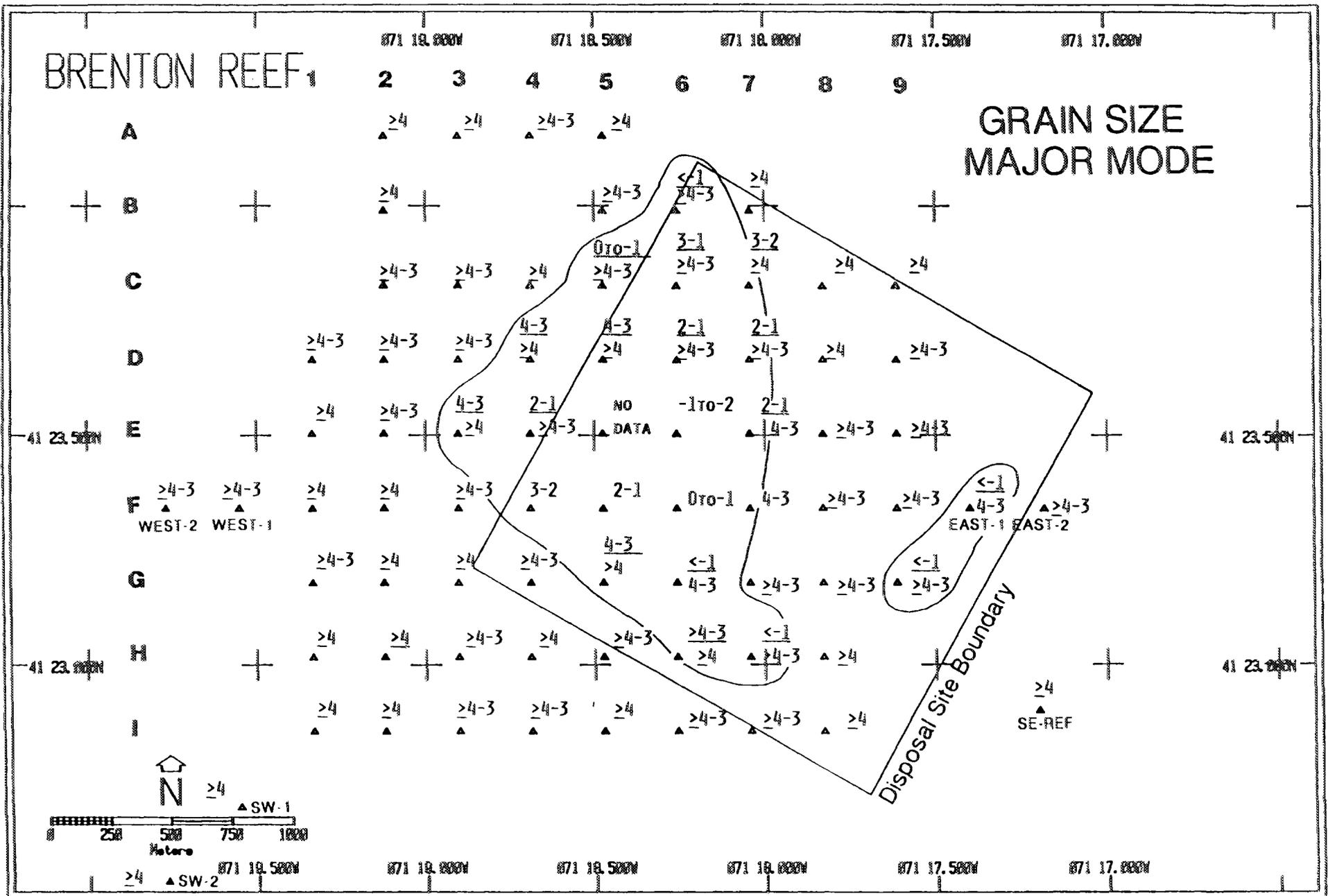
Figure 3-5. Map of grain size major mode (in phi units) of surface sediments at REMOTS<sup>®</sup> stations at the Brenton Reef study site, October 1987. The contours delimit the distribution of dredged material as mapped in Figure 3-4.
