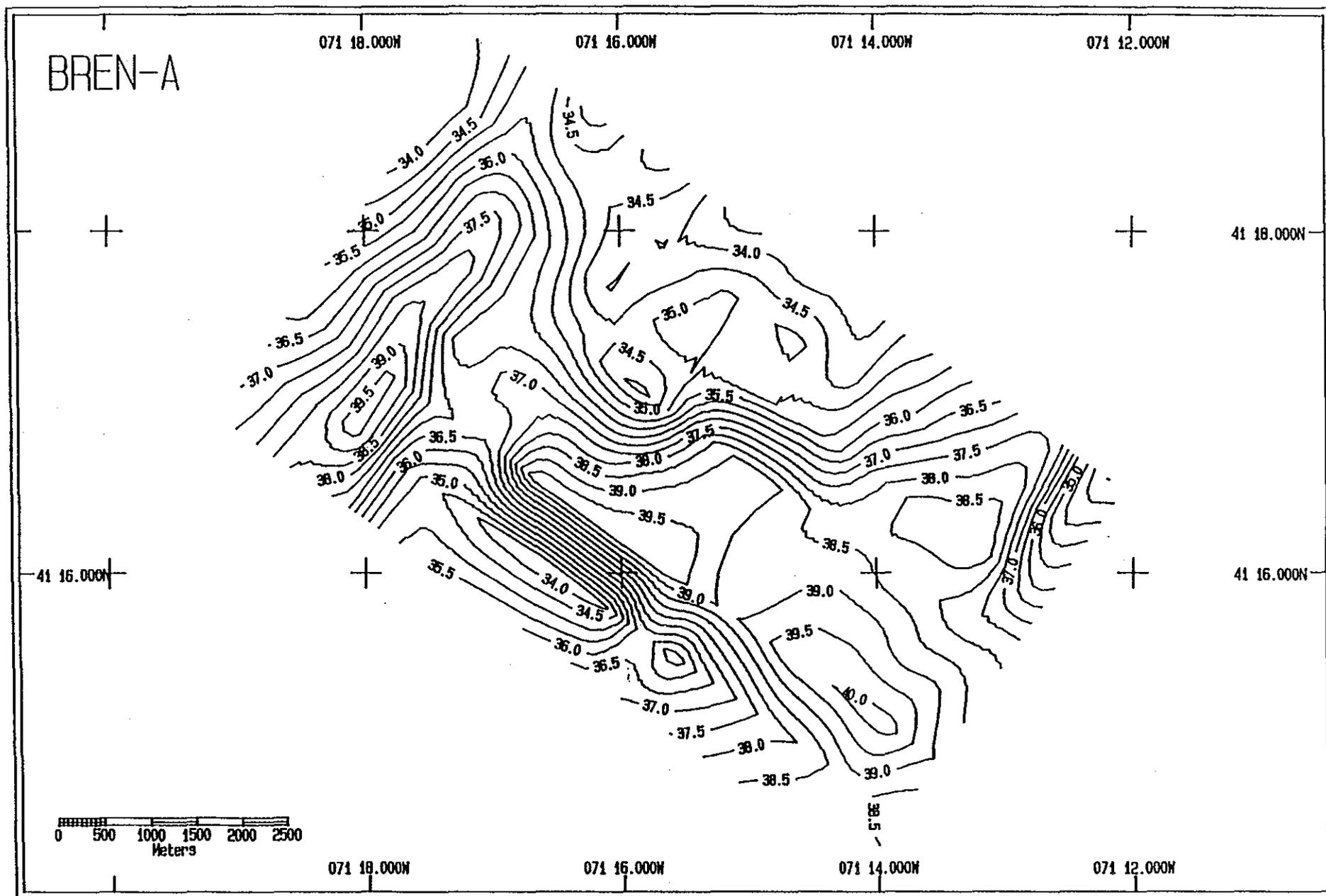
Figure 3-23. Contoured bathymetric chart of the Brenton-A study area, October 1987. Depths are in meters.
