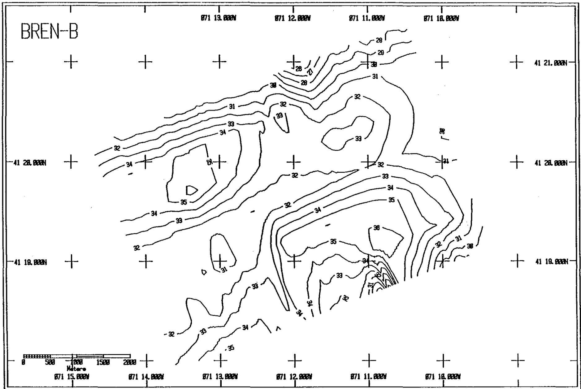
Figure 3-24. Contoured bathymetric chart of the Brenton-B study area, October 1987. Depths are in meters.
