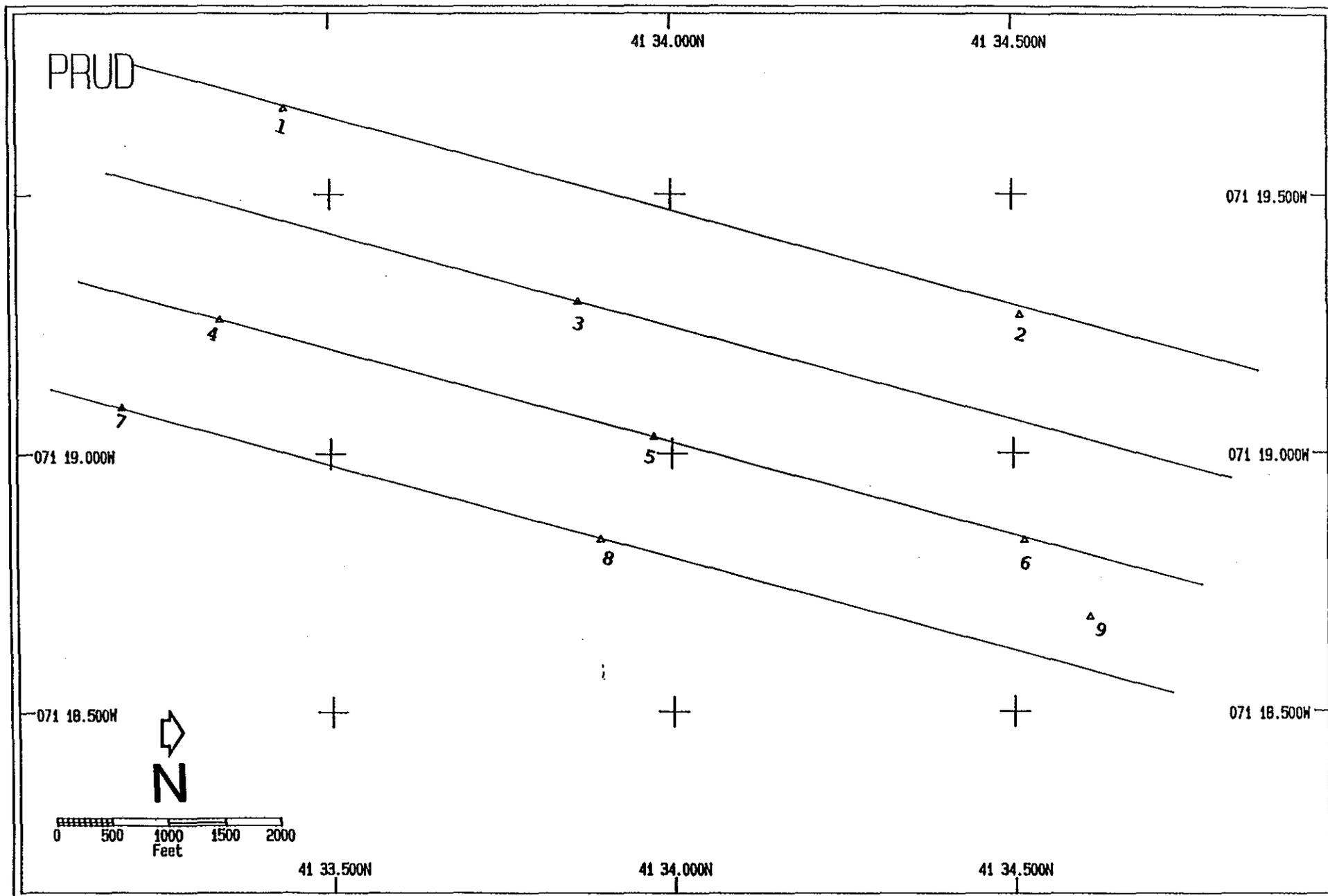
Figure 2-2. Survey lanes for the bathymetric and side-scan surveys at the Prudence study site. The locations and designations of the 9 grab sample stations for visual descriptions and grain size analyses of sediments are indicated by the
