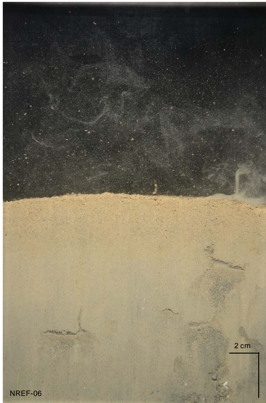
Figure 3-6. The small-scale surface topography (i.e., boundary roughness) in this profile image from station NREF-06 was due to the presence of biogenic mounds created by the burrowing and feeding activities of subsurface organisms
