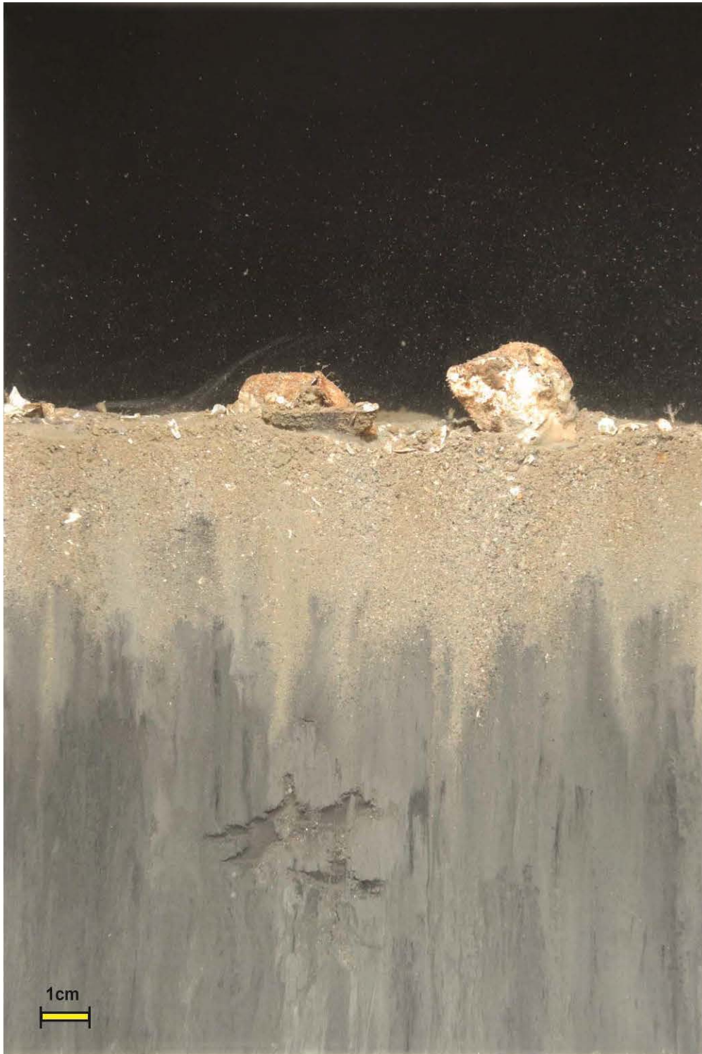
Figure 3-17. Profile image showing sand-over-mud stratigraphy at station 36 located on the 2005 mound
