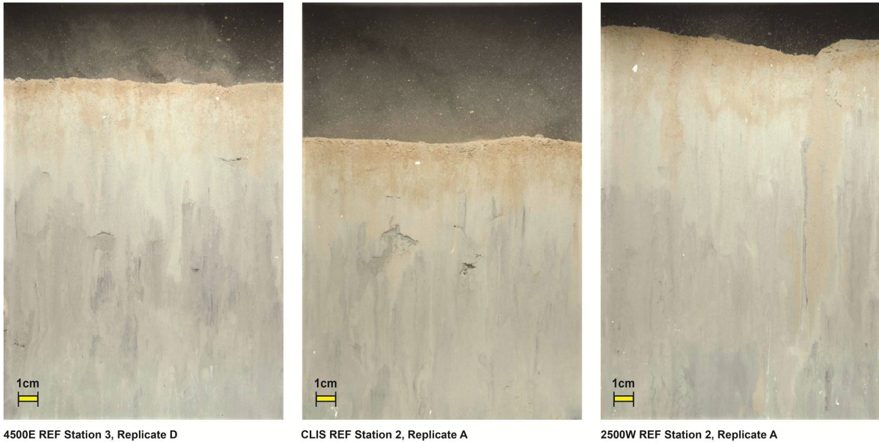
Figure 3-8. Representative profile images illustrating the soft, homogenous mud that characterized each of the three reference areas
