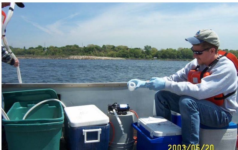
50. Filling sample bottles from the pump system (05/20/2003)
