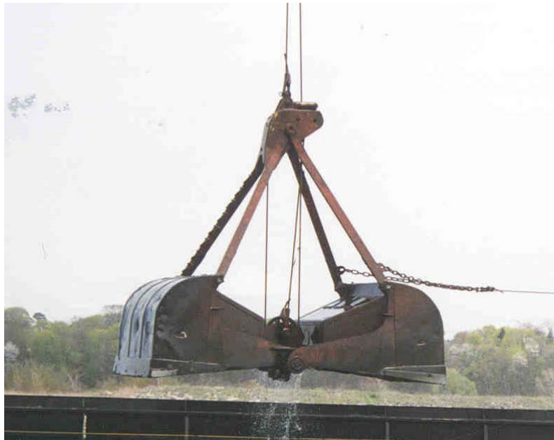
Figure 3-2. Open clamshell bucket (top) and enclosed clamshell bucket (bottom) used on the PRHMDP
