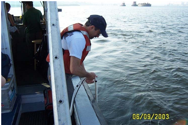
52. Lowering the datasonde/pump intake on station (06/09/2003)
