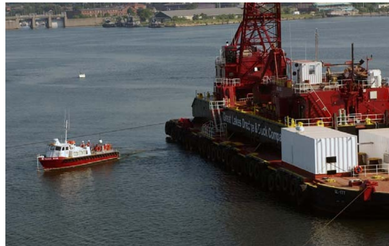
6. Dredge 55 – Positioned over Cell 6/7R, note anchor cables (07/30/2003)
