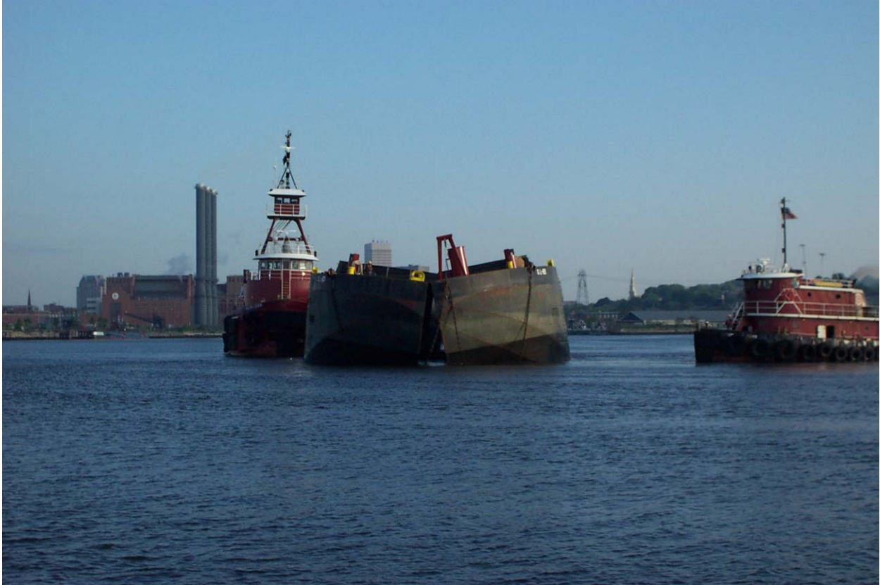
Figure 3-3. Attending tugs with split-hull scow initiating disposal into CAD cell in Providence Harbor
