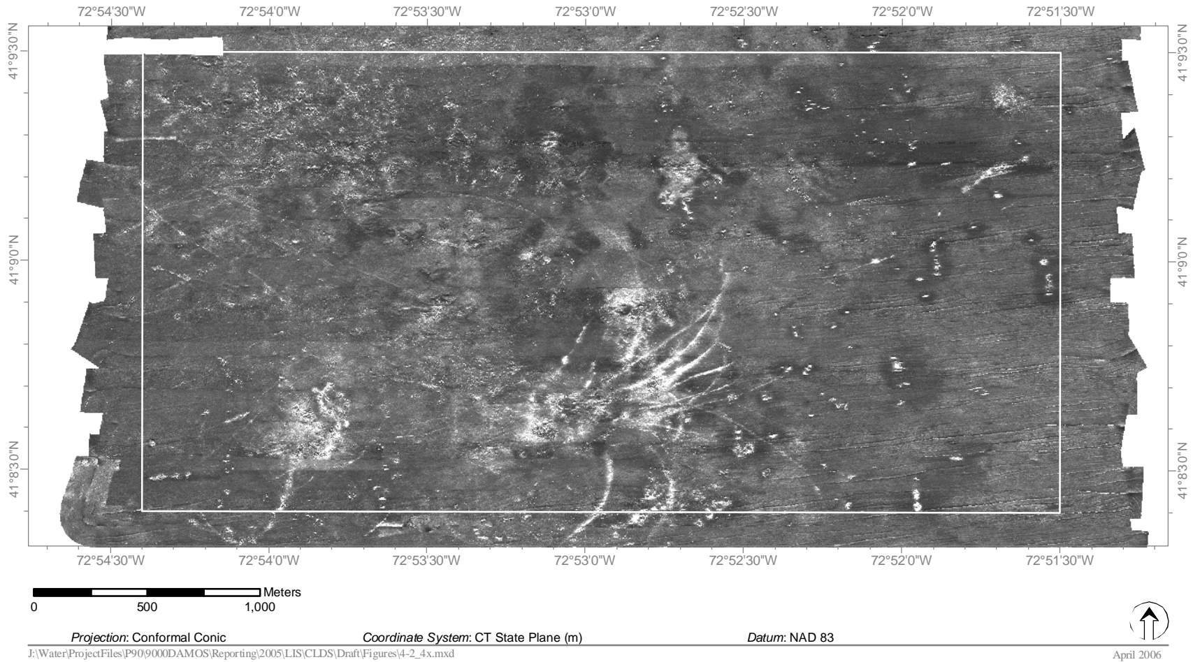
Figure 4-2. U.S. Geological Survey (USGS) side-scan mosaic from 1997 survey. Reprojected to Conformal Conic, CT State Plane, NAD 83 Datum. Histogram stretched from original raster grid to emphasize high backscatter results. Data from Poppe et al. 2000.
