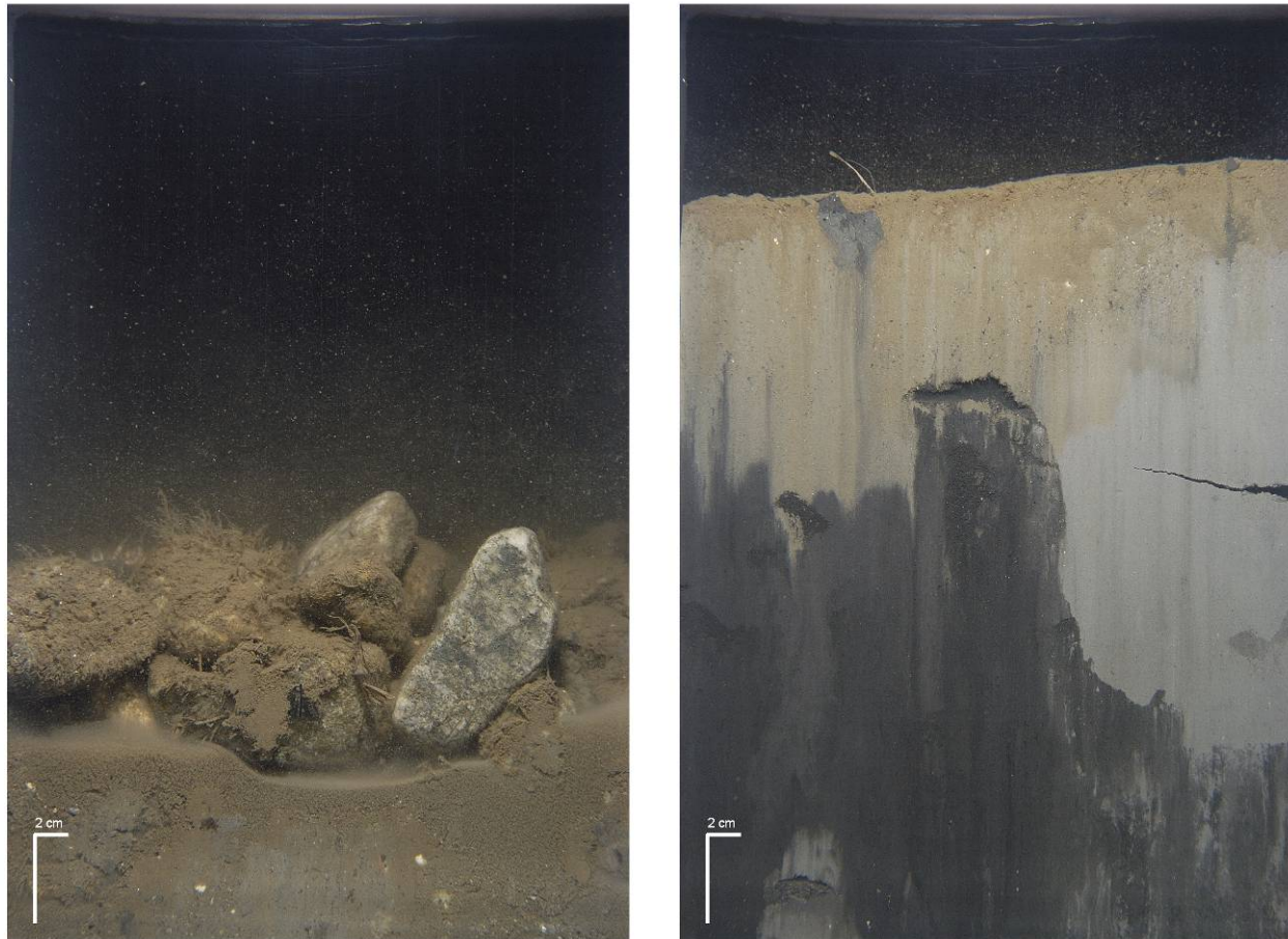
Figure 3-11. Images showing the heterogeneity in sediment type from the recent disposal activities, which affected the camera's prism penetration. The layer of cobbles on top of the fine sediments at Station JH-10 (left) allowed the prism to only penetrate the seafloor an average of 4.3 cm. The recently-deposited muds at Station JH-11 (right) were quickly reworked by burrowing organisms (note feeding void in lower left quadrant), helping to lower sediment shear strength and resulting in a prism penetration mean depth of 18.5 cm.
