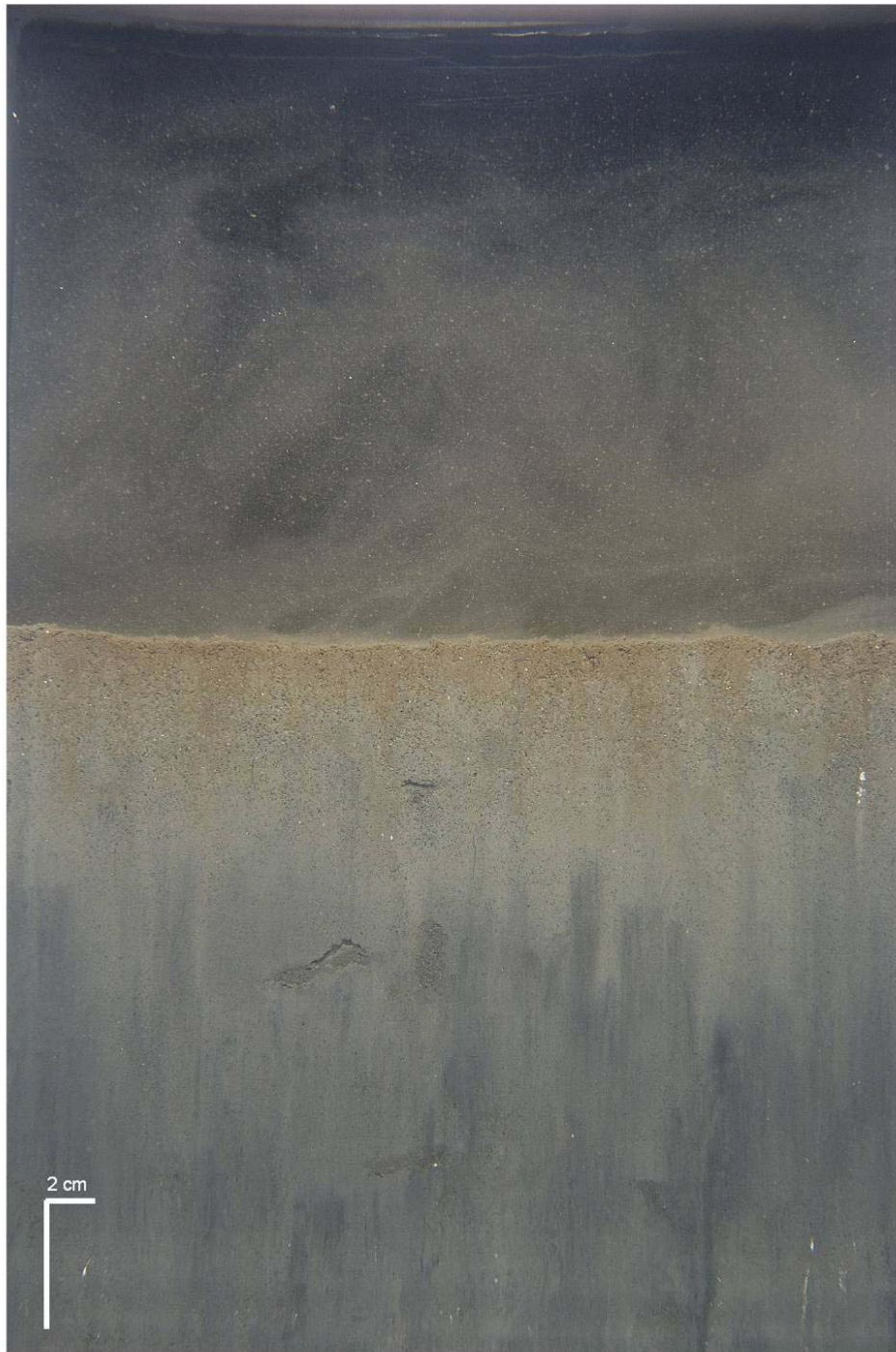
Figure 3-5. Sediment-profile image from Station S-03 showing a surface layer of silty, very fine sand on top of a mud ( \geq 4 phi) facies.
