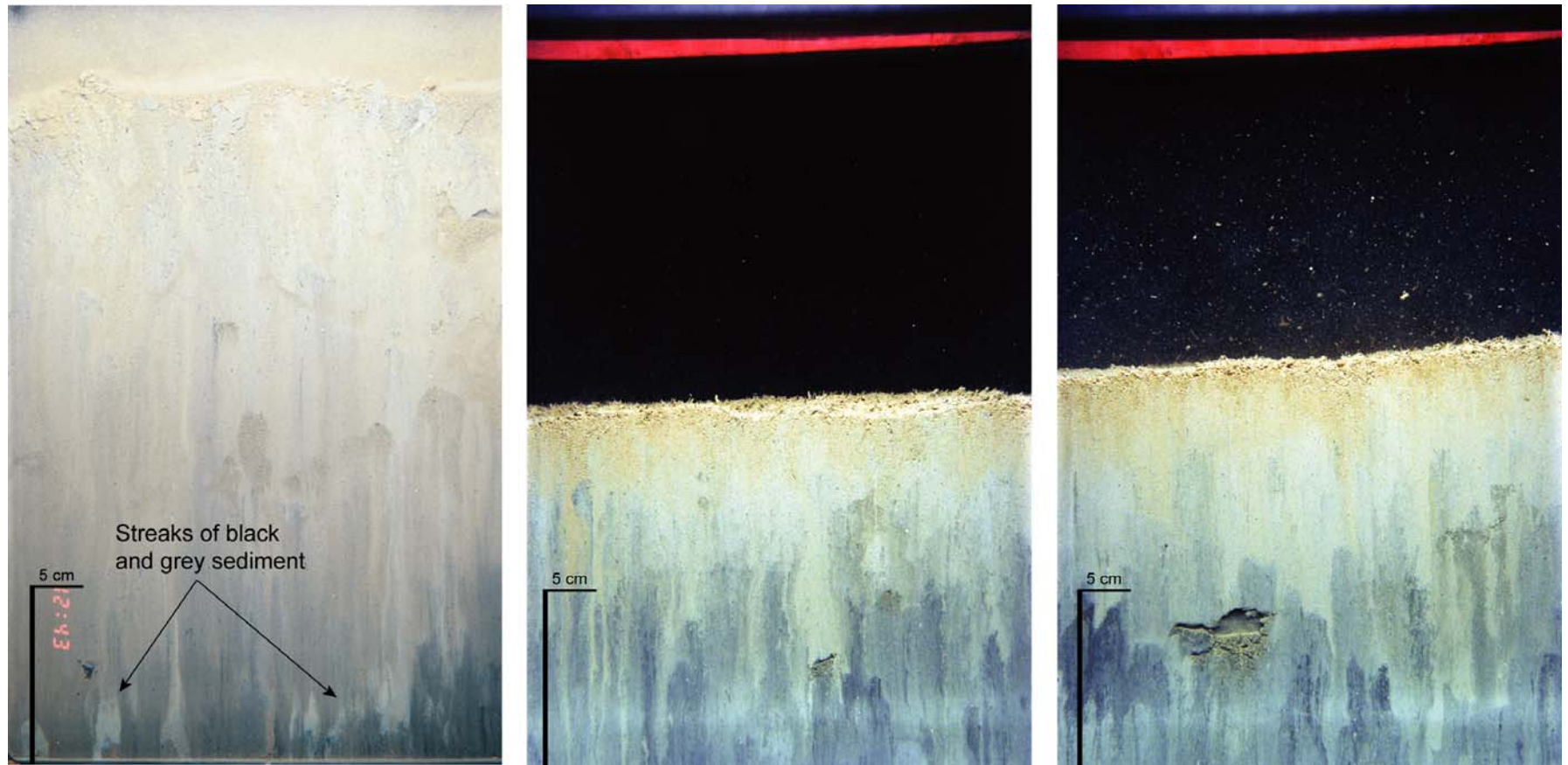
Figure 4-1. SPI images obtained at Station I7 in the September surveys of 2000 and 2003 compared to East Reference Area Station ER2. Deeper penetration of the SPI camera in 2000 (left) revealed streaks of black and gray sediment at depth that were interpreted as evidence of an old dredged material layer exceeding the camera's imaging depth. Such evidence was not observed in the 2003 survey; the sediment at Station I7 (center) appeared similar to the ambient sediment at the reference area (right).
