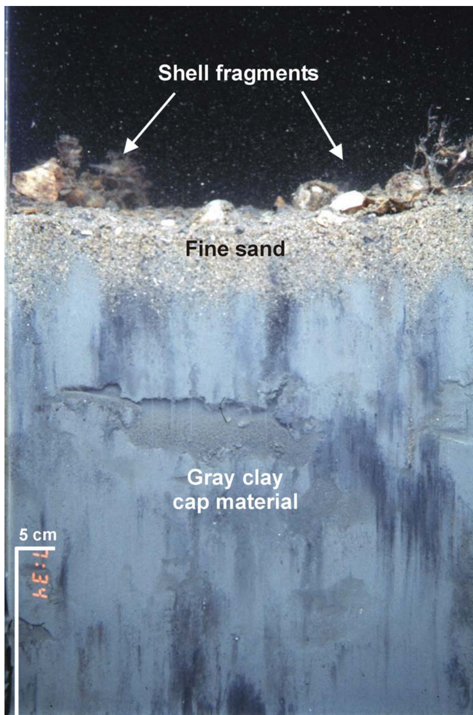
Figure 3-11. REMOTS® image collected from Station 150S displaying a sand over gray clay stratigraphy
