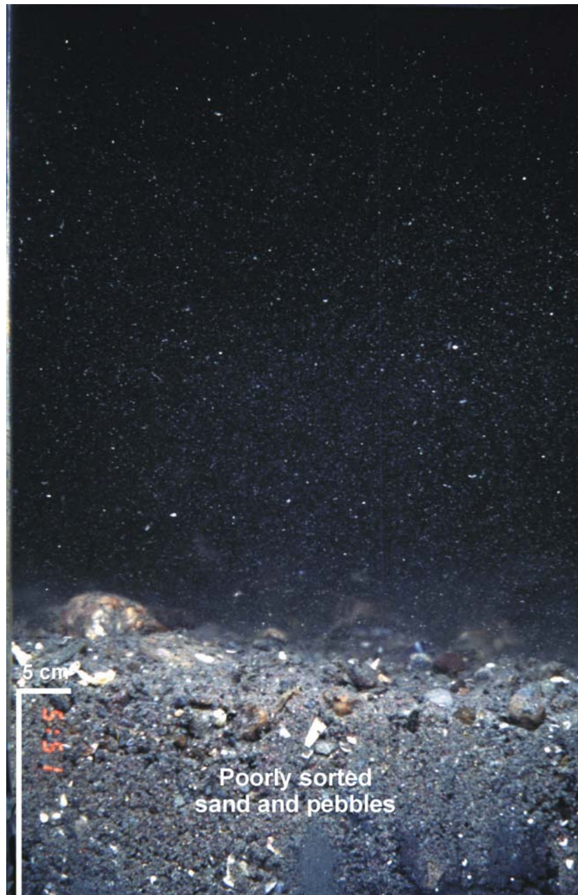
Figure 3-12. REMOTS® image from Station 300E illustrating dredged material comprised of poorly sorted sand and pebbles, likely representative of newly deposited CDM intended for the nearby Dow/Stonington (D/S) Mound. The presence of pebbles and shell hash over finer-grained sediment may suggest some minor small-scale winnowing of the surface sediments.
