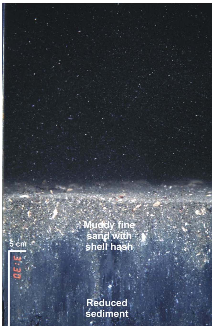
Figure 3-18. REMOTS® image from reference Station WEST-REF5 showing ambient muddy fine sand with considerable amounts of shell hash (grain size major mode of 3 to 2 phi). Reduced sediment is visible at sediment depth.
