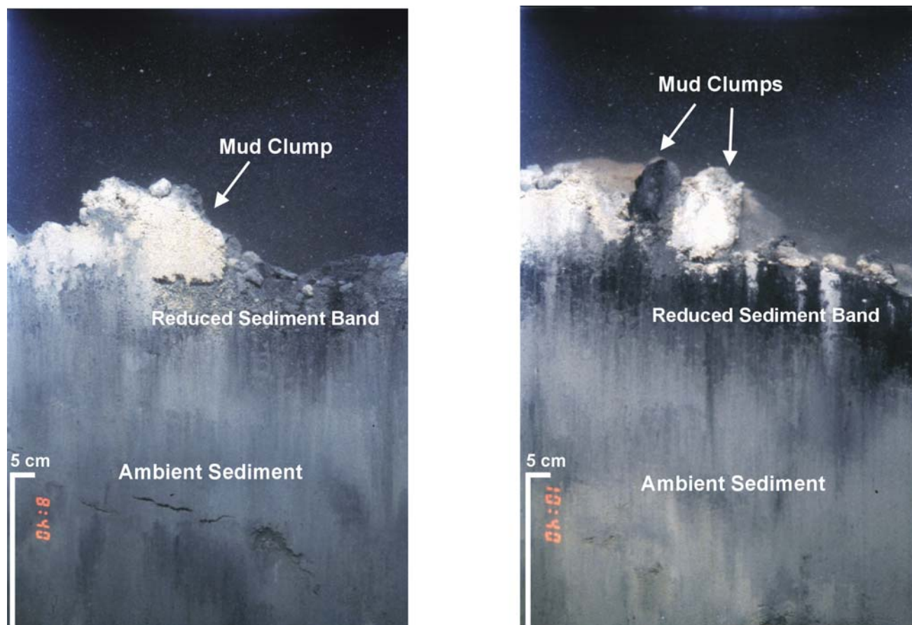
Figure 3-8. REMOTS ® image from outer station O04 (left) and TLDS reference area station WREF3 (right) displaying cohesive mud clumps at the sediment surface. Horizontal bands of black, sulfidic sediment are also visible near the sediment surface.
