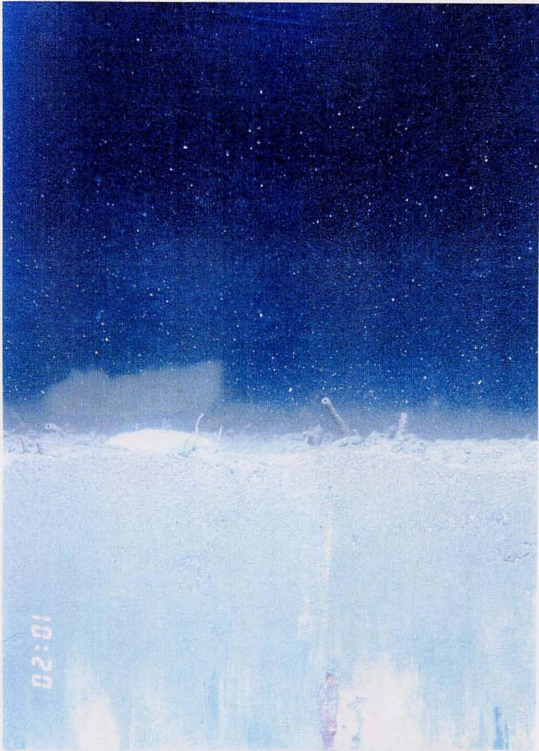
**Figure 3-3.** Layer of biogenically reworked sediments over dredged material and large Stage III polychaete feeding in the dredged material layer
