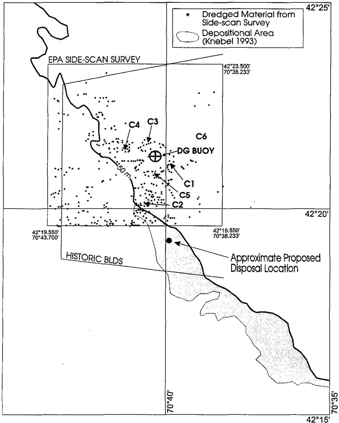
**Figure 1-2.** The relative locations of dredged material located by side-scan sonar (Schoenherr et al. 1992); 1994 REMOTS® sampling transects; a depositional sedimentary environment above the 50 m depth contour (Knebel 1993); and a proposed disposal location (Normandeau Associates 1994)
