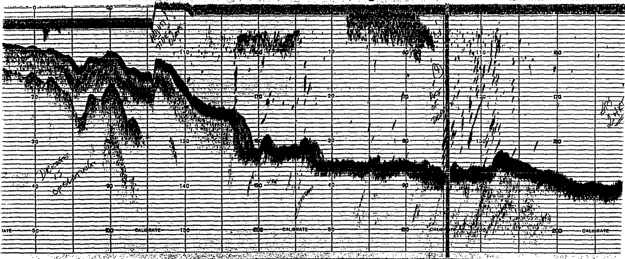
Beginning segment of Transect B acoustic profile surveyed on 25 October 1993; profile runs east to west
