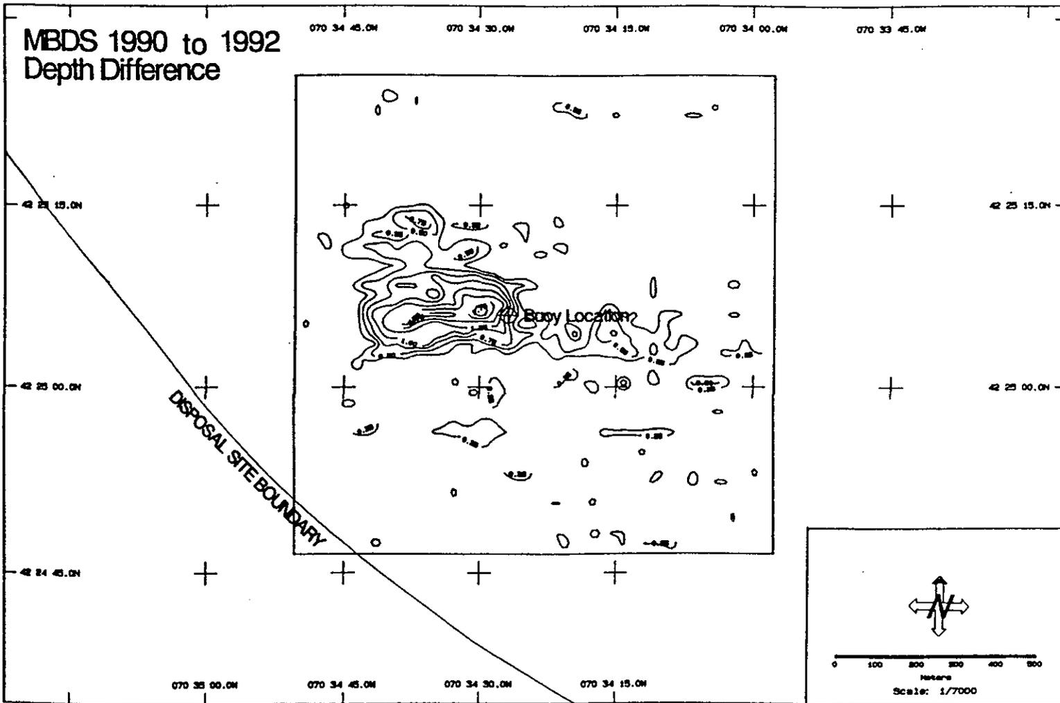
Figure 3-3. Contoured depth difference chart (in meters) at MBDS from 1990 to 1992. The contour interval is 0.25 m.
