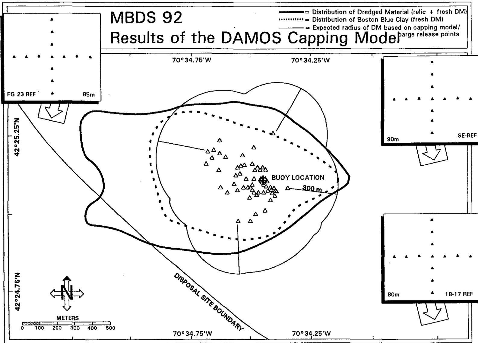
**Figure 4-5.** Expected radius of dredged material distribution based on barge release points (September 1990 to March 1992) and the DAMOS capping model
