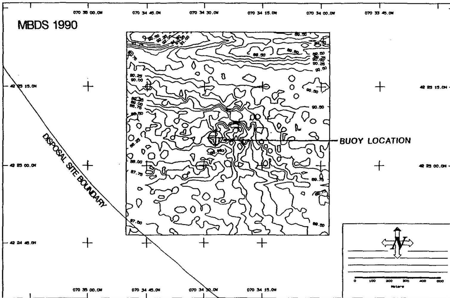
Figure 3-2. Contoured bathymetry chart (depth in meters) of MBDS, August 1990. The contour interval is 0.25 m.
