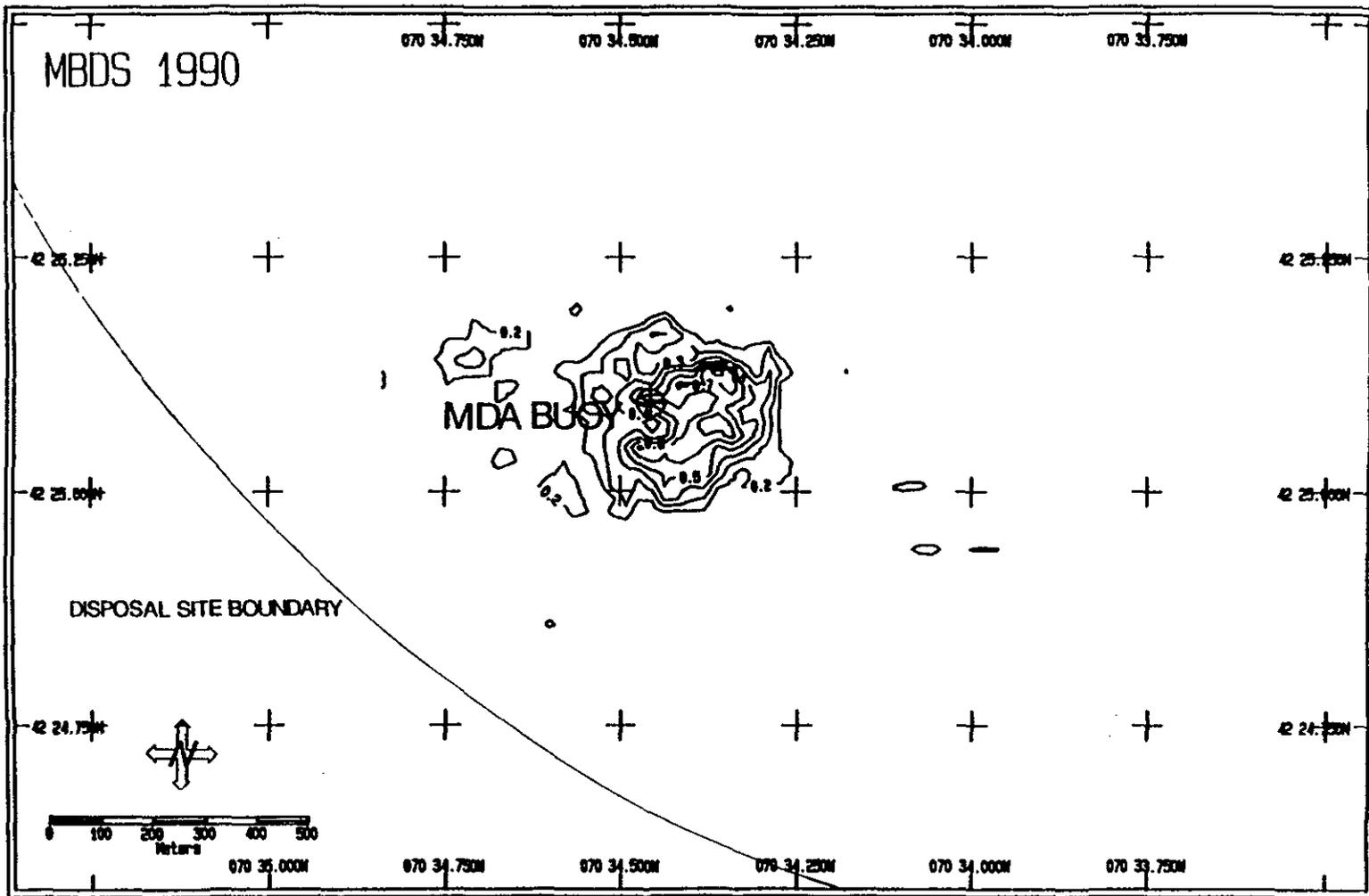
Figure 4-2. Contoured depth difference chart (in meters) at MBDS from 1988 to 1990. The contour interval is 0.25 m.
