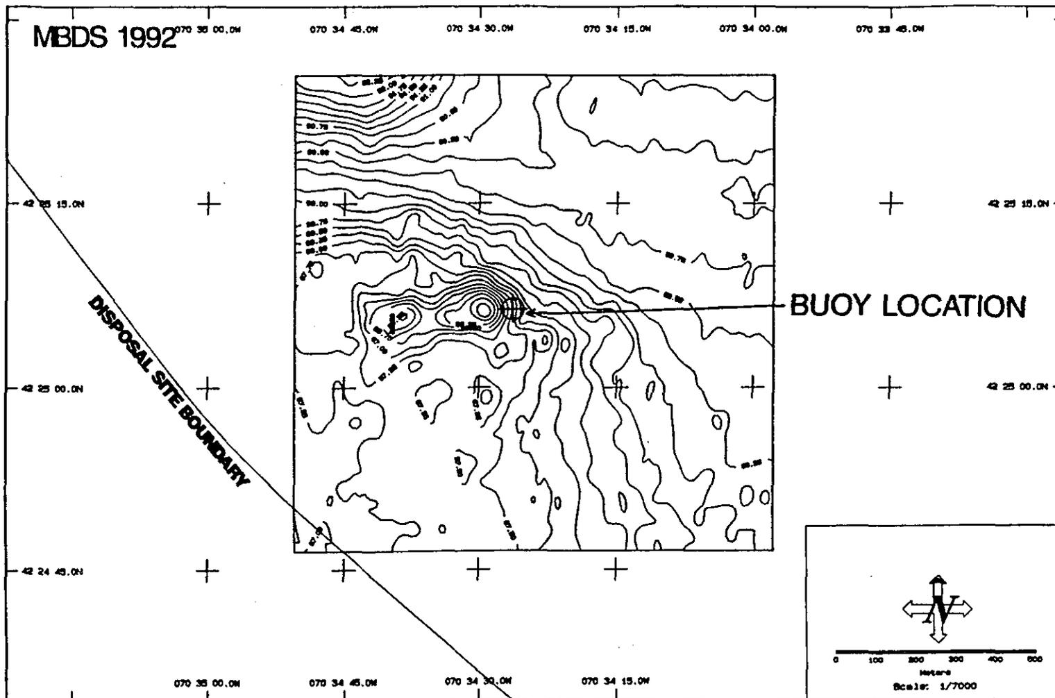
Figure 3-1. Contoured bathymetry chart (depth in meters) of MBDS, 31 March 1992. The contour interval is 0.25 m.
