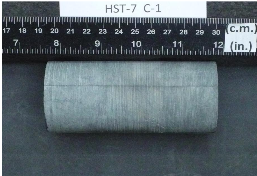
After cutting and grinding
