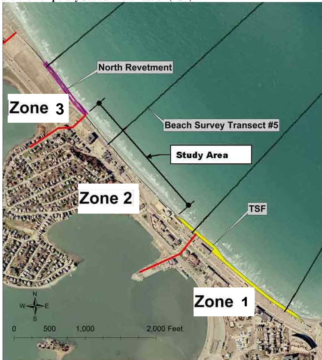
Figure 1 Nantasket Beach Zone 2 Study Area located between the North Revetment and the Temporary Seawall Fortification (TSF)
