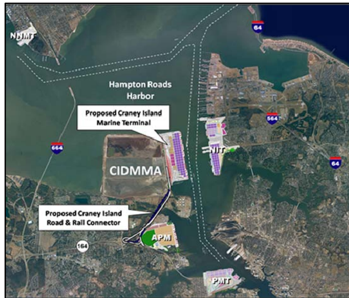
Figure 2.2-3. Craney Island eastward expansion project schematic.
