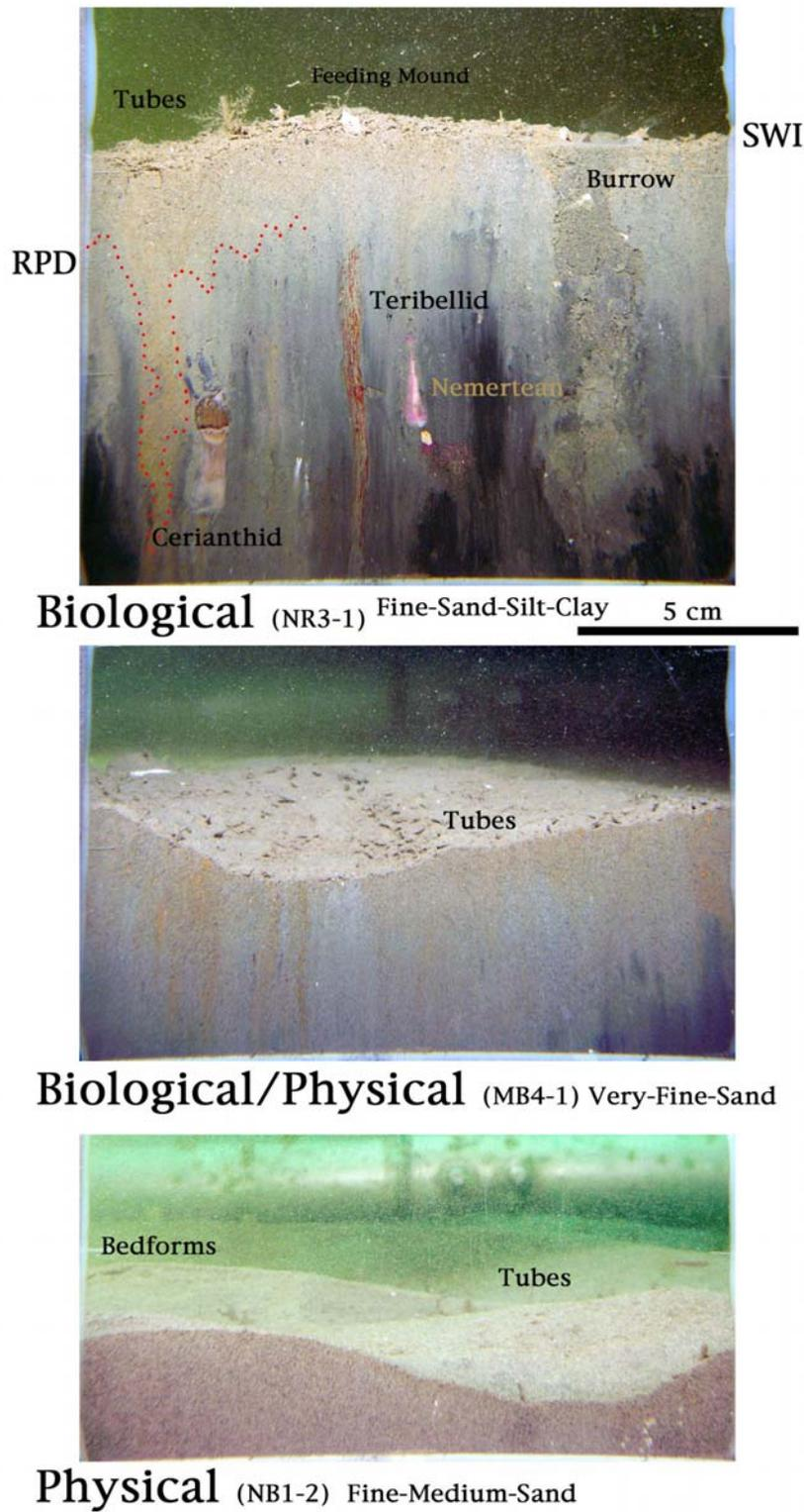
**Figure 8. Example Images of Sediment Surfaces Dominated by Physical and Biological Processes and Sediment Types Encountered within the Five Regions of Interest. SWI is sediment-water-interface.**
