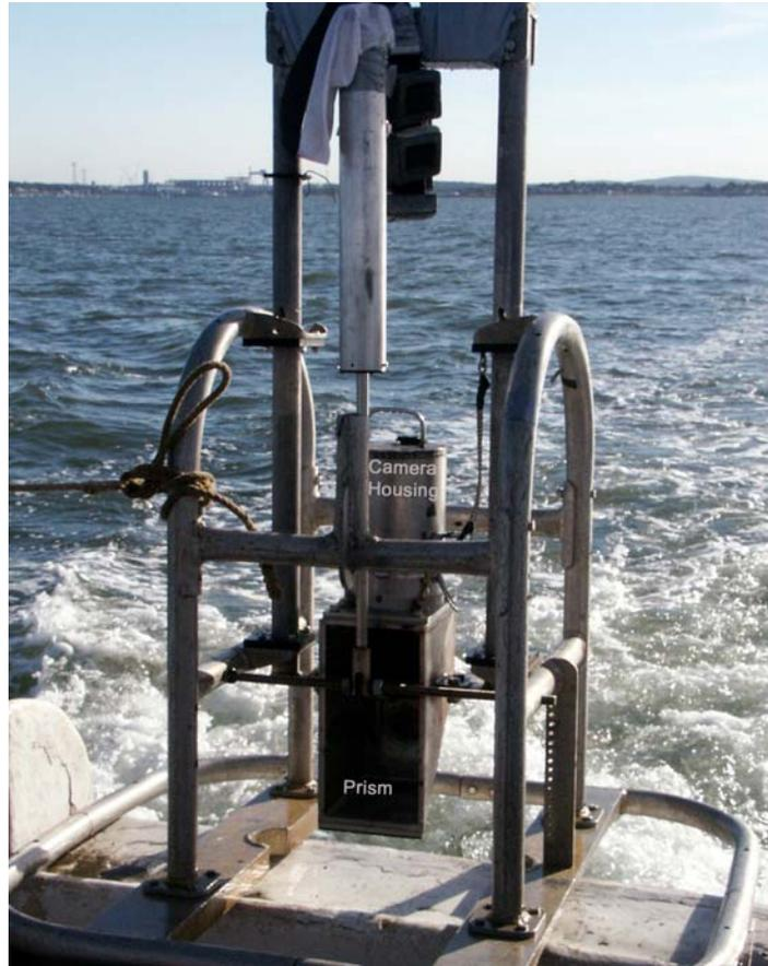
**Figure 2. Sediment Profile Camera, Width of Prism is 15.5 cm.**
