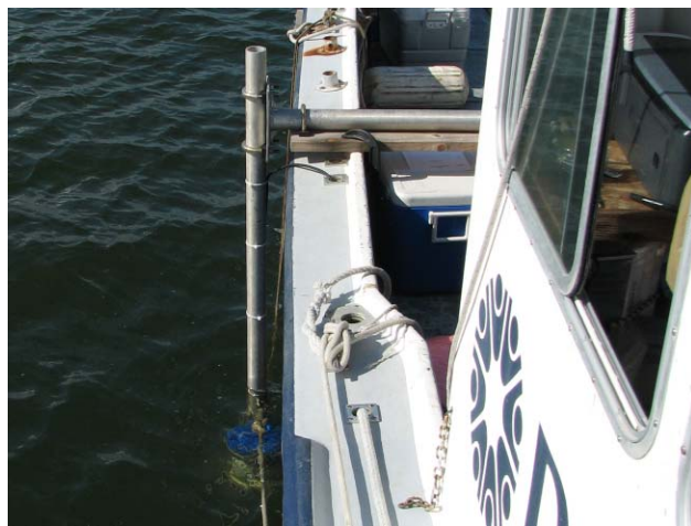
Figure 6. ADCP Mounted in Operational Position Over the Side of the Aquamonitor with the Acoustic Transducers Just Below the Water Surface.
