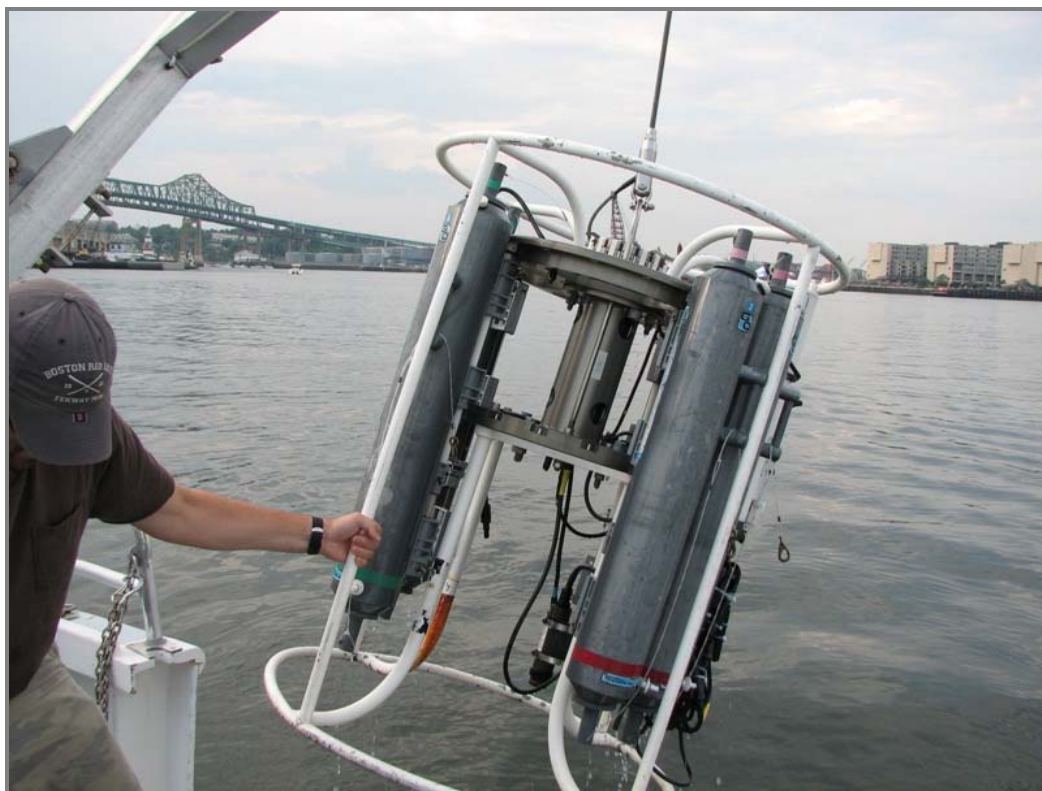
Figure 9. CTD/Turbidity/Dissolved Oxygen Profiler and Water Sample Rosette System Being Deployed from the R/V Aquamonitor .
