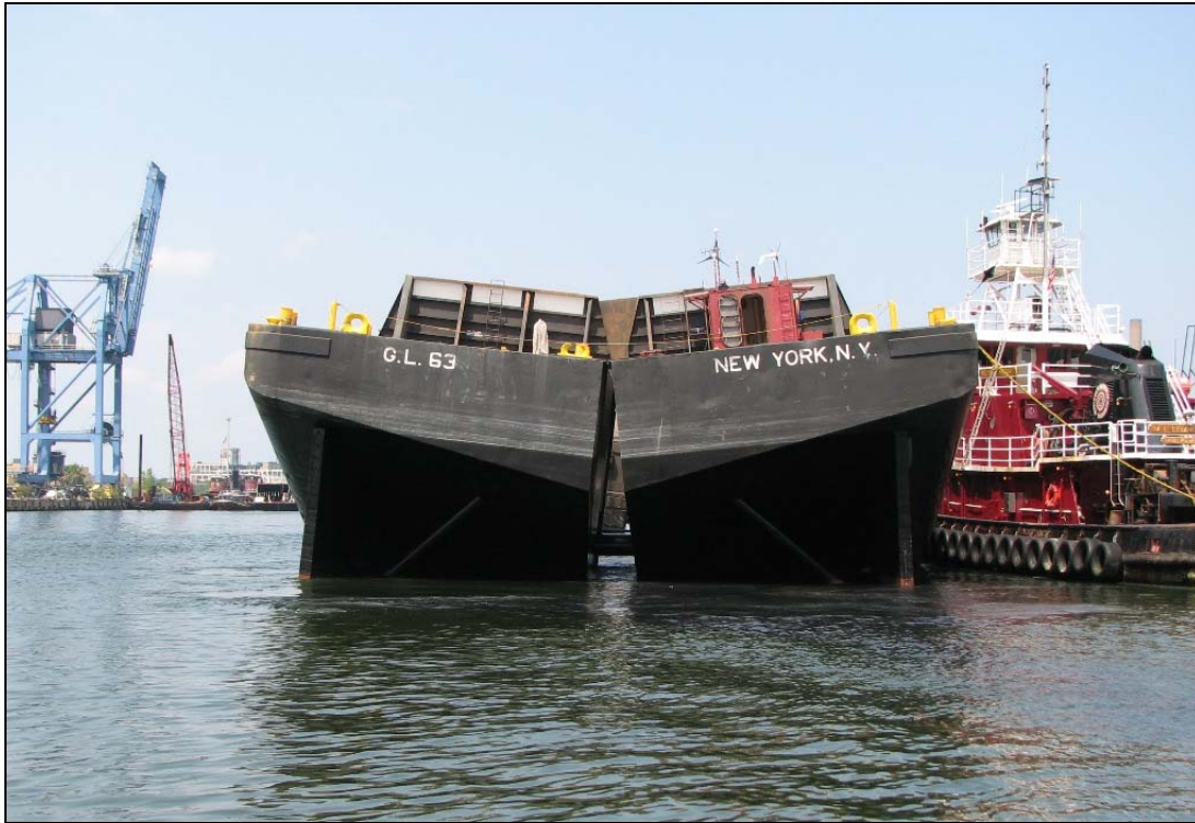
Figure 8. Split Hull Scow Immediately after Placement of Dredged Material into the Mystic River CAD Cell.
