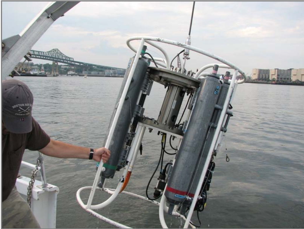
Figure 4. CTD/Turbidity/Dissolved Oxygen Profiler and Water Sample Rosette System Being Deployed from the R/V Aquamonitor .
