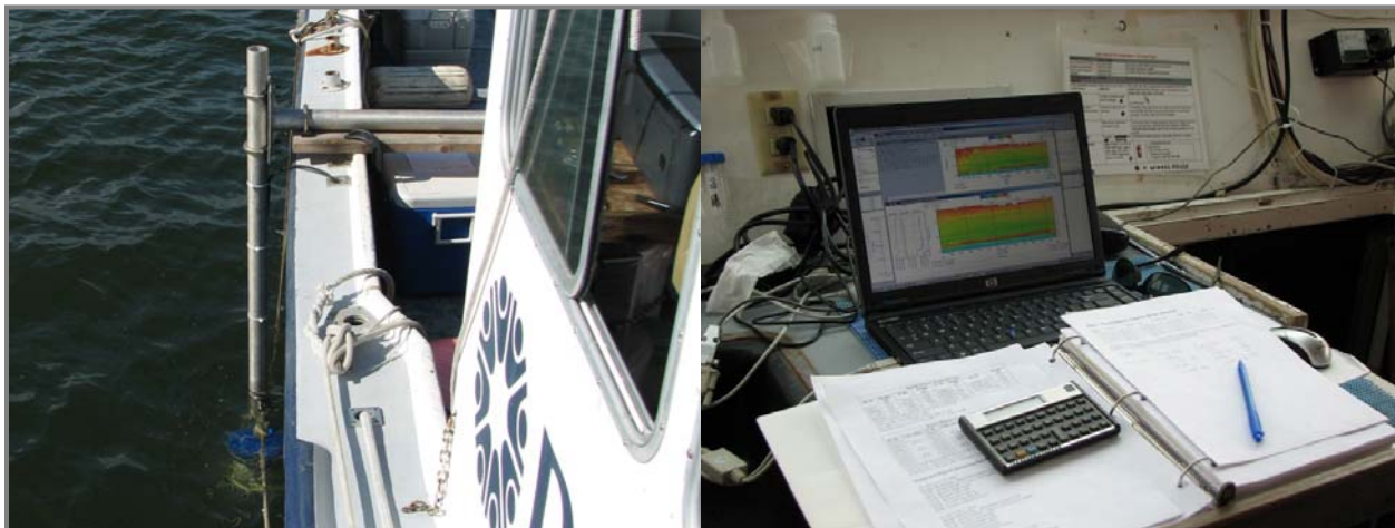
Figure 4. RD Instruments 1200kHz Workhorse Sentinel ADCP Mounted on the Battelle R/V Aquamonitor and ADCP Real-Time Display / Data Collection laptop.
