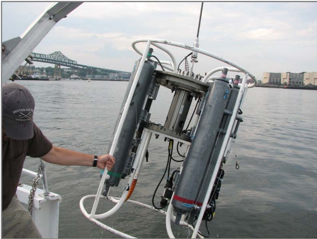
Figure 5. CTD/Turbidity/Dissolved Oxygen Profiler and Water Sample Rosette System Being Deployed from the R/V Aquamonitor.
