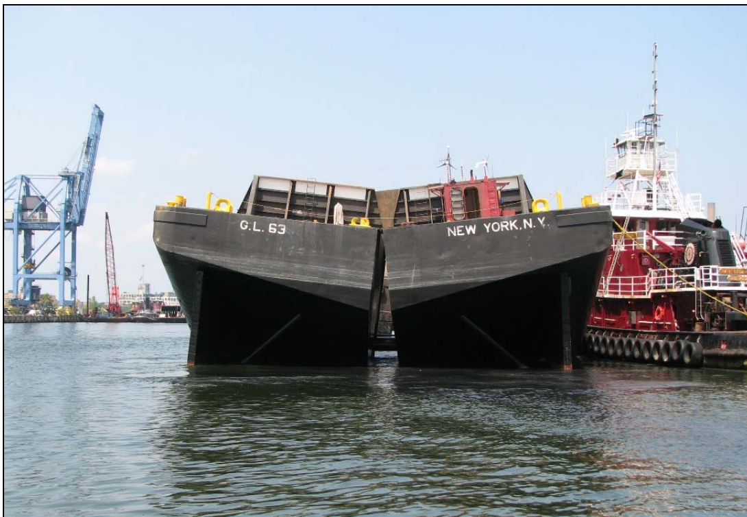
Figure 3. Split Hull Scow Placing Dredged Material into the Mystic River CAD Cell.
