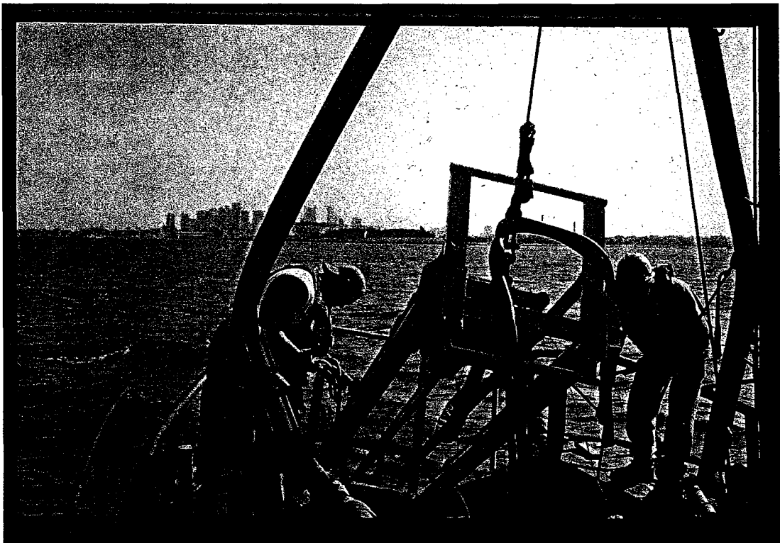
Figure 5. Vibratory core mechanism being raised. Boston skyline in background.
