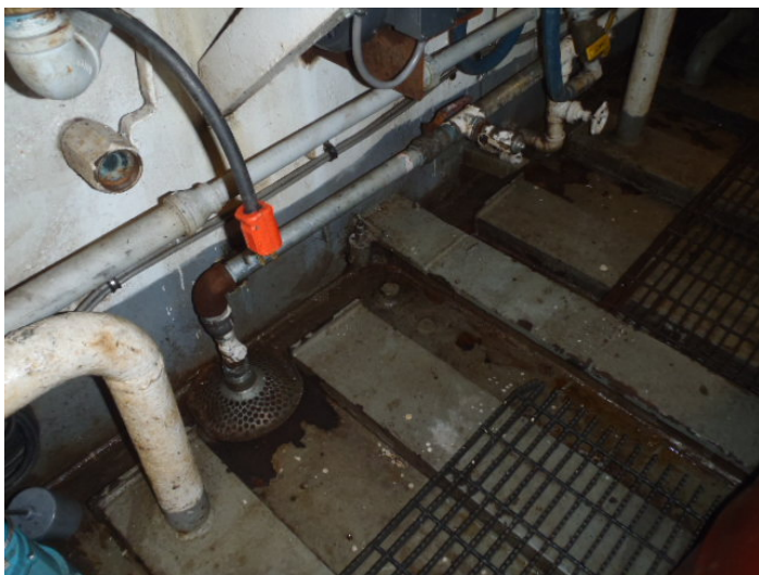
Fixed bilge suction – internal channel keel coolers – portable bilge pump
