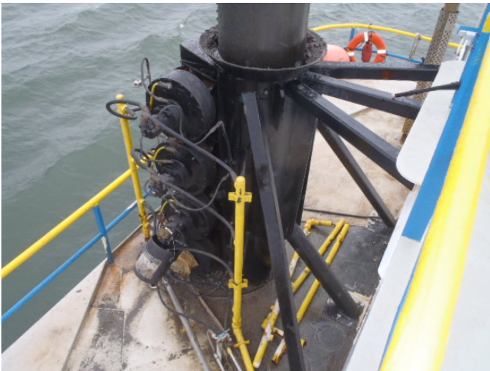
Four hydraulic motors per leg
