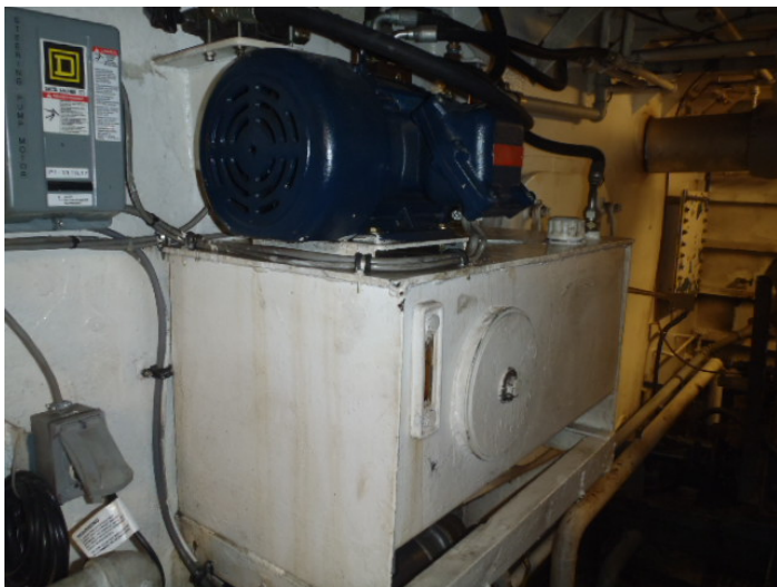
Electro hydraulic steering system
