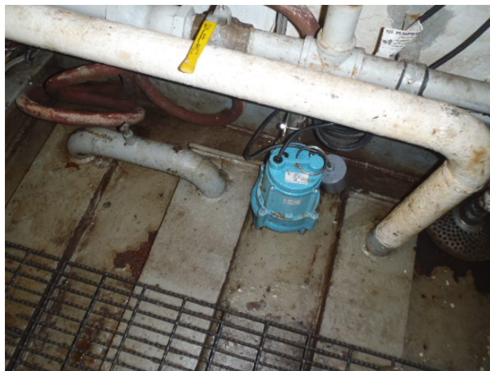
Fixed bilge suction – internal channel keel coolers – portable bilge pump
