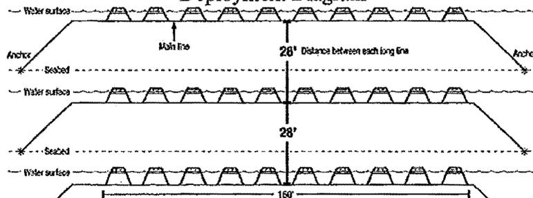
A typical long line consists of one individual row of 10 to 12 OysterGro Units. The units are linked together with 3/8" ropes. Proper anchorage is necessary to hold the units to the seabed. The long lines are usually around 160 feet.
