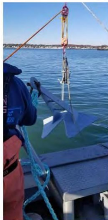
Photo #5: A 200-pound embedment anchor suspended and waiting to be deployed
