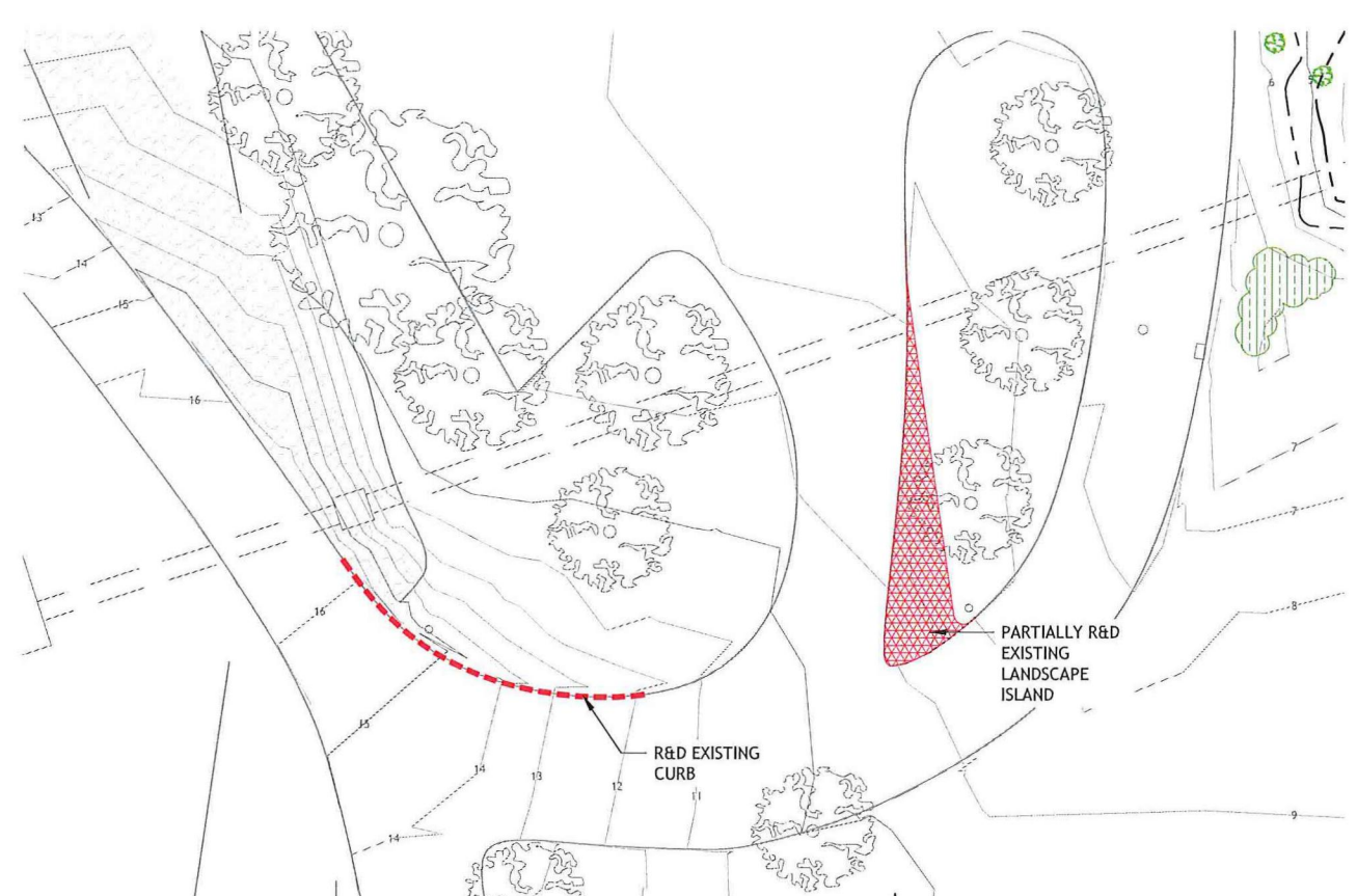
ROAD WIDENING DEMO PLAN SCALE: 1"=20'-0"
