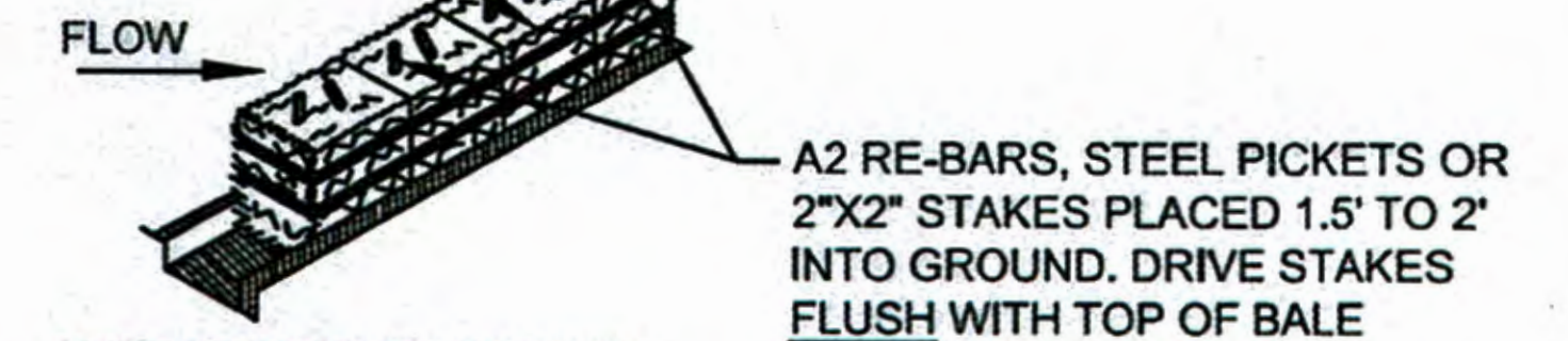
ANCHORING DETAIL SINGLE-STACKED STRAW BALE DIKE DETAIL NOT TO SCALE
