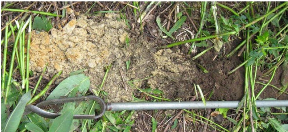
Plot F2 Soil Profile: High contrast between depleted soil matrix and masses within the C-horizon
