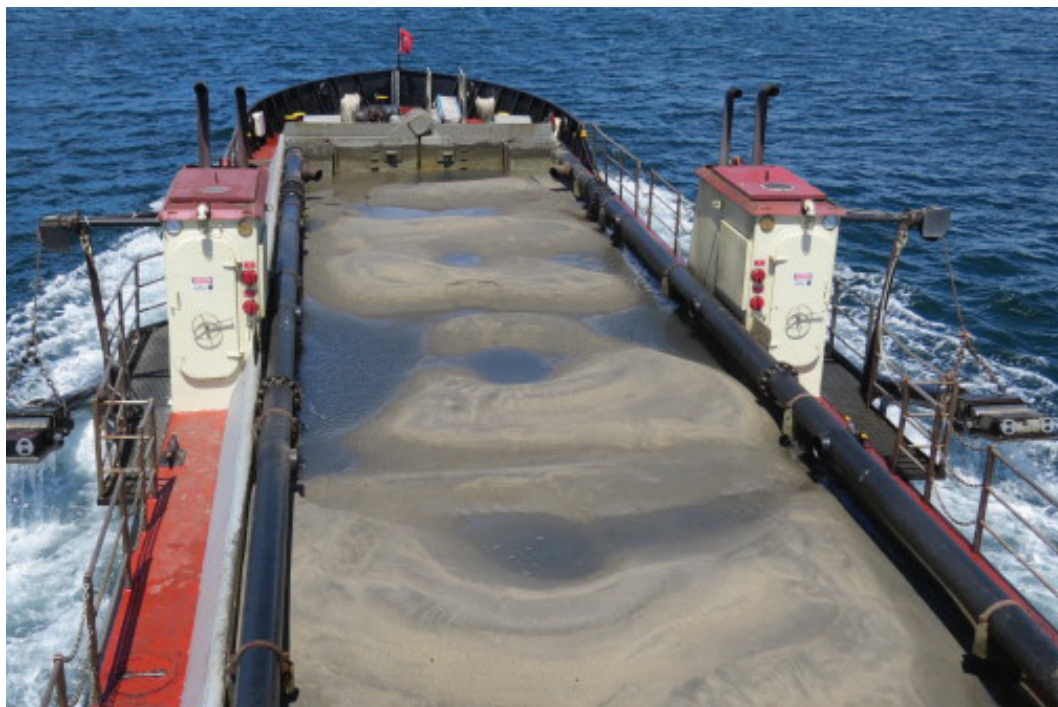
The CURRITUCK drains the water, leaving only material behind.
