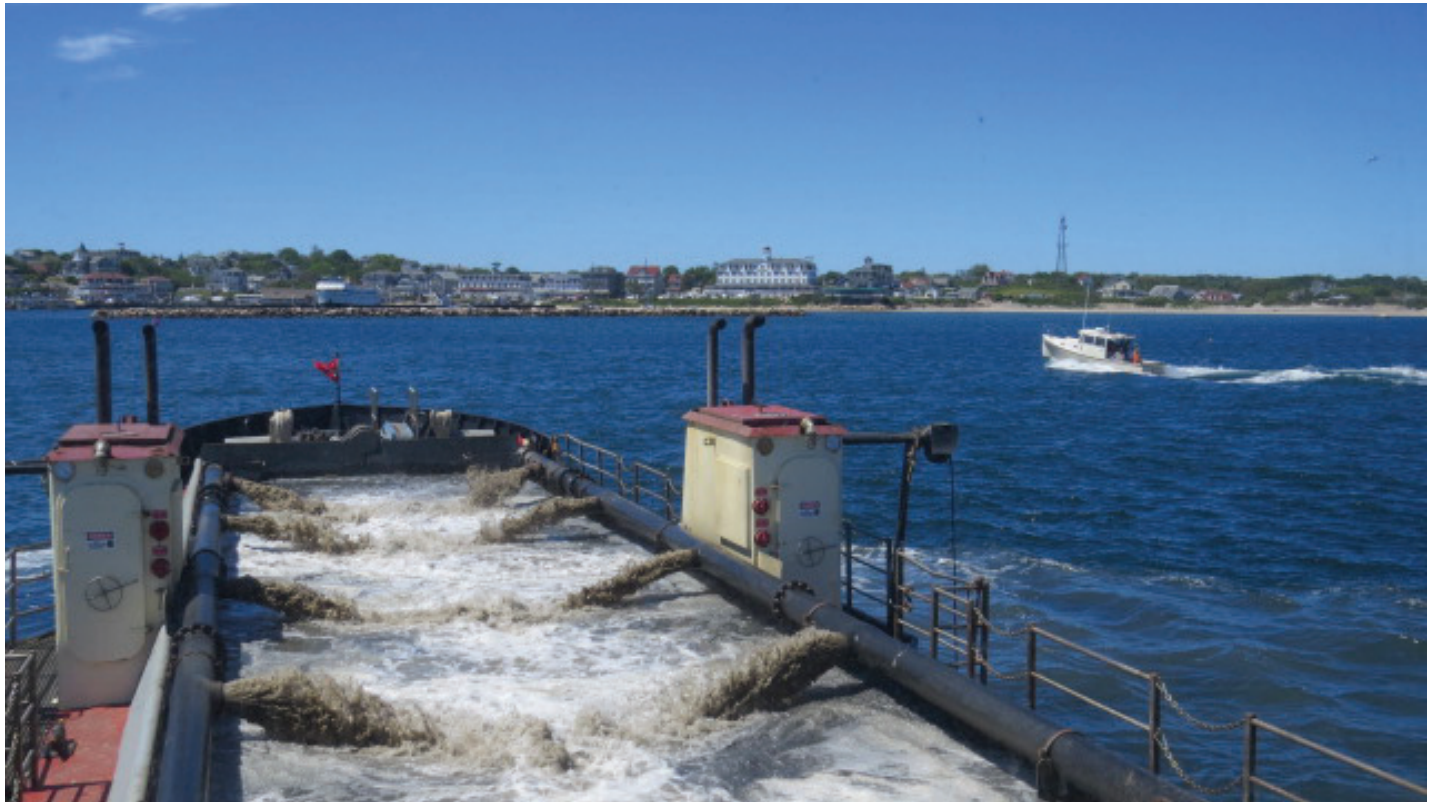
The CURRITUCK fills with water and material during the dredging process.
