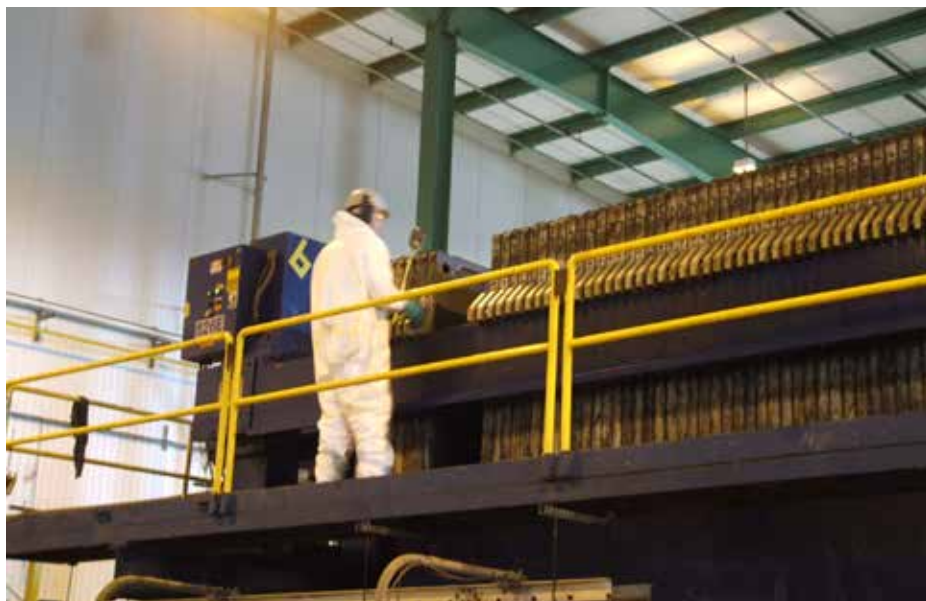
Contractor inspecting a filter press at the New Bedford Superfund Site.
