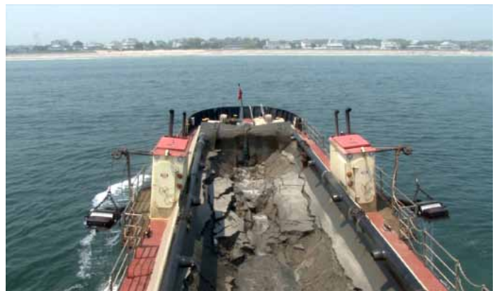
The CURRITUCK opens the hull and deposits sediment at the disposal site.
