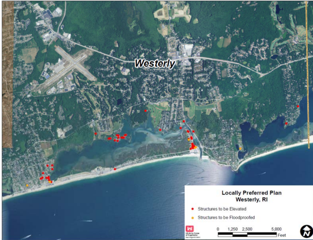
Figure E9: Alternative 6, Westerly Structure Locations
