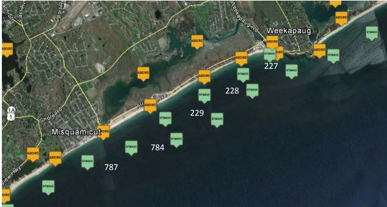
Figure 6-3. ADCIRC save point stations from the NACCS study (accessed through the CHS)
