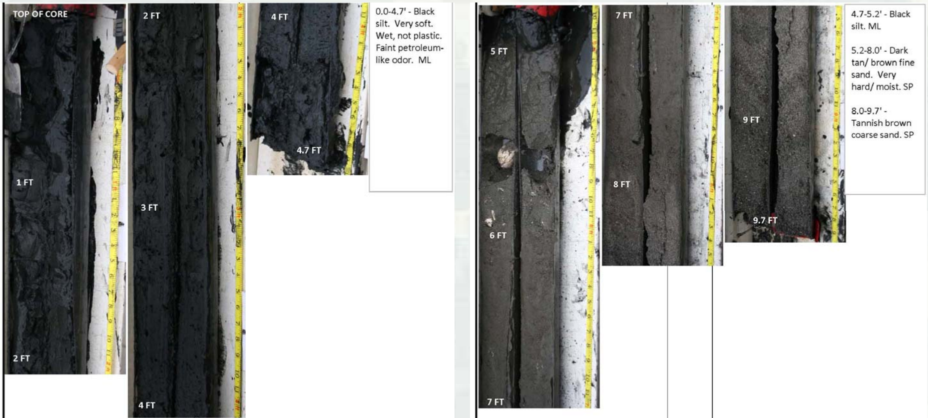
Core Log from Station X – material type = silt and clay from sediment-water interface to 5.2 ' / silty sand below
