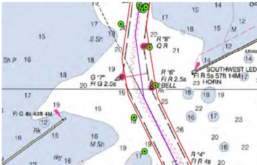
Figure 4 - Proposed New Haven Federal Navigation Channel Bend Widening
