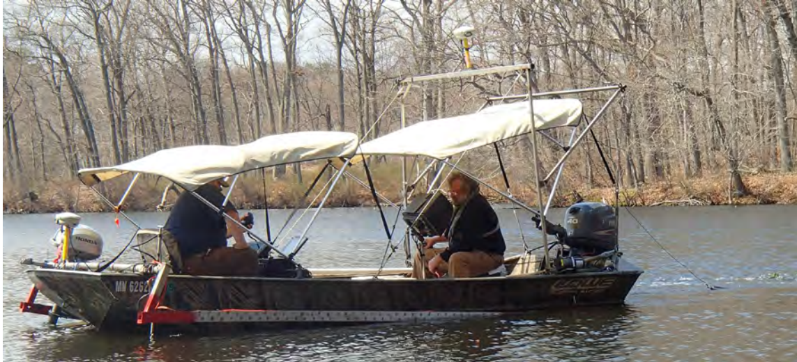
17-ft Jon boat on which Side-scan Sonar and Bathymetry Equipment will be deployed
