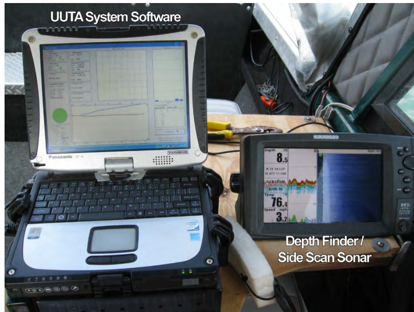
UUTA control systems and data displays
