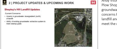
Andy Vitolins presented the SHL updates. This slide shows SHL, the cap, Plow Shop Pond to the east, Nonacoicus Brooke to the north, and the groundwater extraction system at the north end of the landfill. Current concerns here are arsenic in groundwater downgradient (north) of the landfill and the ability of the existing groundwater treatment system to meet the cleanup goals for arsenic.
