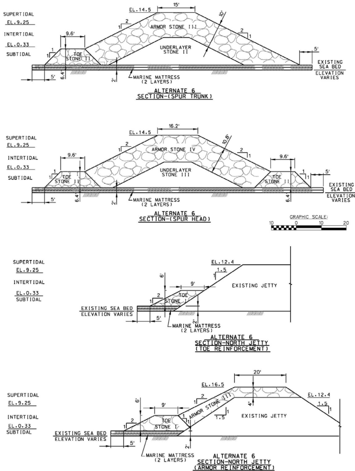
**Figure 3-1 – Cross-Section of Spur Jetty and North Jetty**
