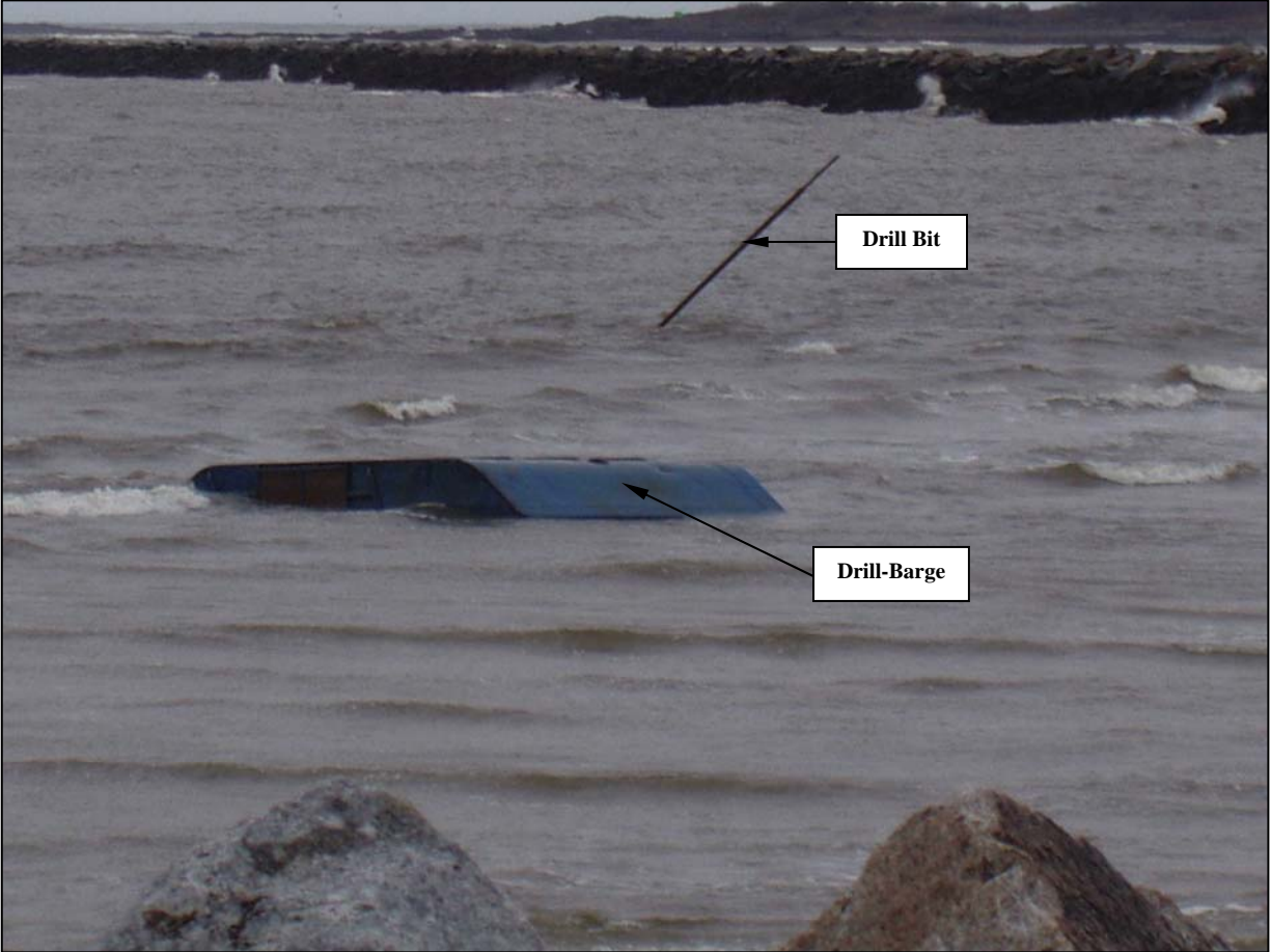
Figure 5-3. Sunken modern geotechnical boring drill-barge and displaced drill bits within the Camp Ellis Beach project survey area (source: NAE 2009).
