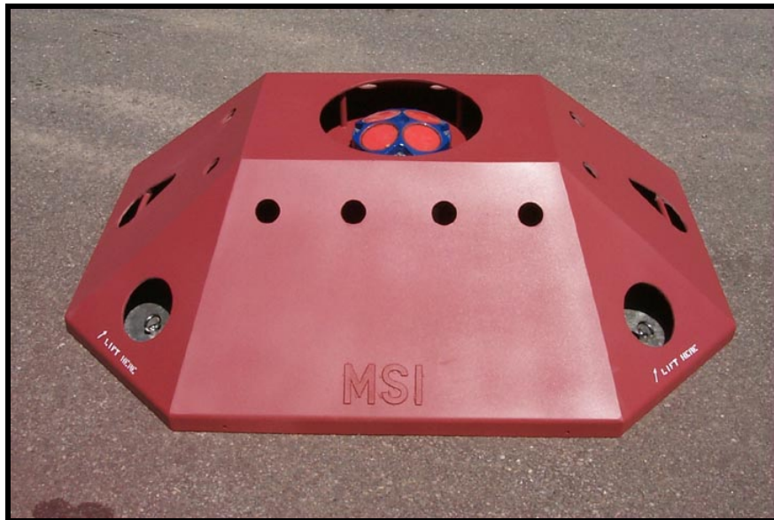
Figure 7-2. ADCP fitted in trawl-resistant bottom mount.
